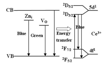
Figure 1.11 Schematic diagram for the mechanism of visible emission from Ce-doped ZnO. [105]
