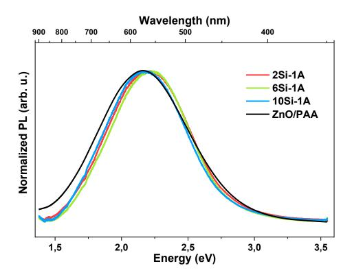
Figure 4.7 Normalized PL spectra of silica-coated ZnO/PAA with different amount of TEOS loading.
