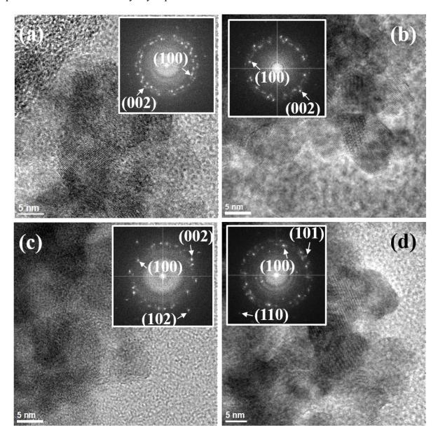
**Figure 3.4** HRTEM images of (a) 0.1 % Mn, (b) 5 % Mn, (c) 0.1 % Cu(II) and (d) 0.1 % Bi doping, showing nanocrystals of ZnO. The insets are FFT images of each HRTEM image, indexed to wurtzite ZnO polycrystalline structure, respectively. More HRTEM images of these samples can be found in Appendix II.
