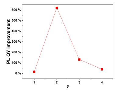
**Figure 4.16** PL QY improvement of 3.8Si-yA silica-coated ZnO nanohybrids compared to their respective uncoated ZnO/PAA precursor in function of the ratio of NH<sub>4</sub>OH *y* in solution A.
