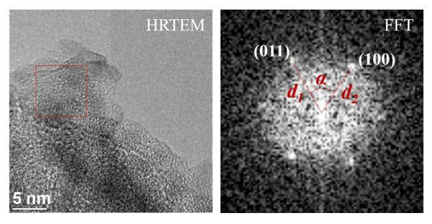
Figure 2.7 Structure indexing via fast Fourier transform (FFT) in HRTEM image.
