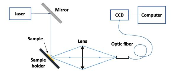
Figure 2.10 PL spectroscopy experimental setup
