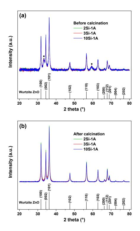
**Figure 4.4** XRD spectra of *x*Si-1A (x = 2, 3 and 10) ZnO nanohybrids (a) before calcination and (b) after calcination at 400 °C for 4 h.
