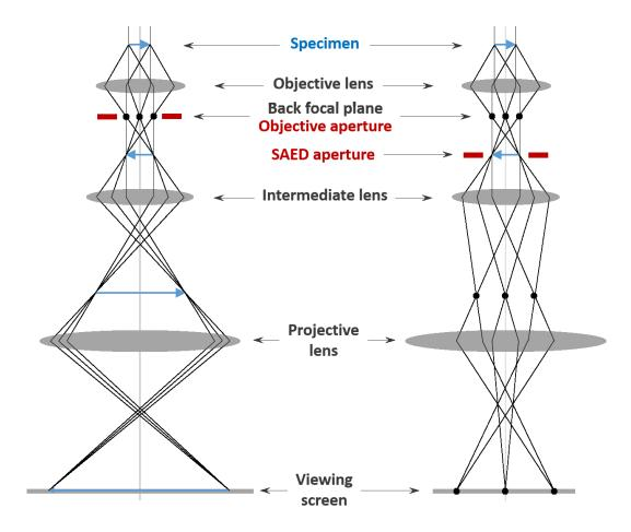
Figure 2.6 Schemes of imaging mode (left) and diffraction mode (right) of TEM.
