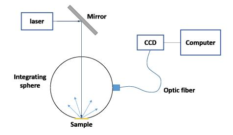
Figure 2.13 Schematic of the setup for PL QY measurements.
