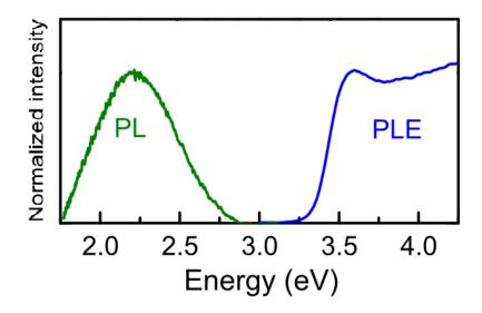
**Figure 2.11** Typical PLE spectrum (in blue) of ZnO along with its PL spectrum (in green).  $\lambda_{em} = 577$  nm,  $\lambda_{ex} = 266$  nm. [195]
