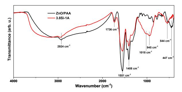
Figure 4.6 FTIR spectra of ZnO/PAA and 3.8Si-1A nanohybrids.
