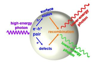
Figure 1.16 Illustration of the mechanism on the origin of the visible emission in ZnO nanocrystal.
