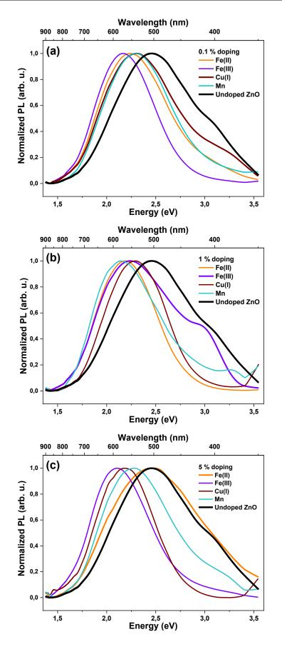
**Figure 3.13** PL spectra of undoped ZnO nanohybrid and Fe(II)-, Fe(III)-, Cu(I)-, and Mn-doped ZnO nanohybrids at (a) 0.1 %, (b) 1 %, and (c) 5 % doping concentrations.
