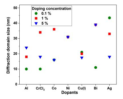
**Figure 3.11** Diffraction domain size of doped ZnO nanonhybrids estimated by Scherrer equation in function of dopants and doping concentration. The dopants are arranged in the ascending order of the ionic radius.
