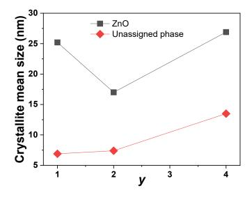
**Figure 4.10** Diffraction domain size of ZnO (squares) and the unassigned phase (diamonds) of three silica-coated samples (3.8Si-yA (y = 1, 2, and 4)) in function of the amount of NH<sub>4</sub>OH in solution A. The size of the unassigned phase is estimated by Scherrer equation from the peak at  $2\theta = 33.4^{\circ}$ .
