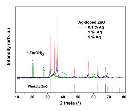
Figure 3.9 XRD spectra of Ag-doped ZnO nanohybrids.
