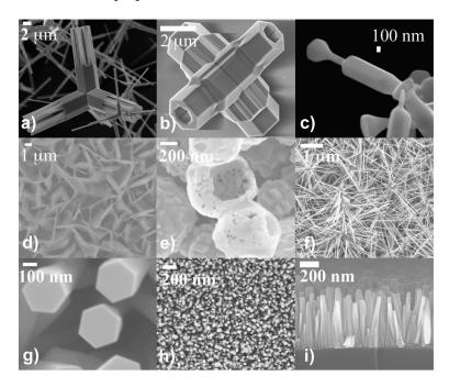
**Figure 1.15** Various morphologies of ZnO nanostructures: (a) and (b) tetrapod structures; (c) variable diameter structures; (d) nanosheets; (e) nanoshells; (f) multipods; (g), (h), and (i) nanorods. [120]
