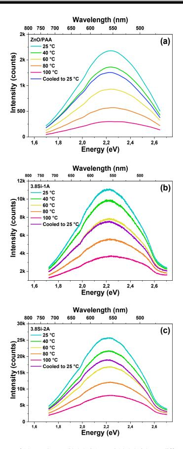
**Figure 4.18** PL spectra of (a) ZnO/PAA, (b) 3.8Si-1A and (c) 3.8Si-2A at different temperatures from 25 °C to 100 °C.
