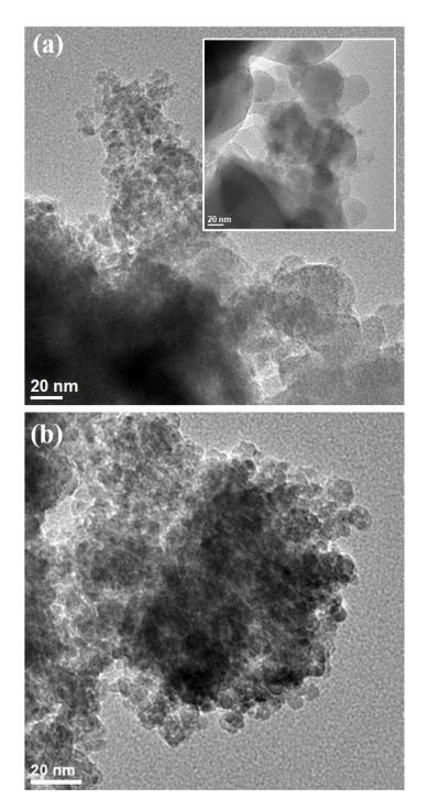
**Figure 3.2** Morphologies of ZnO nanohybrids doped with different elements at 0.1 %. (a) Cu(II) doping. (b) Bi doping.
