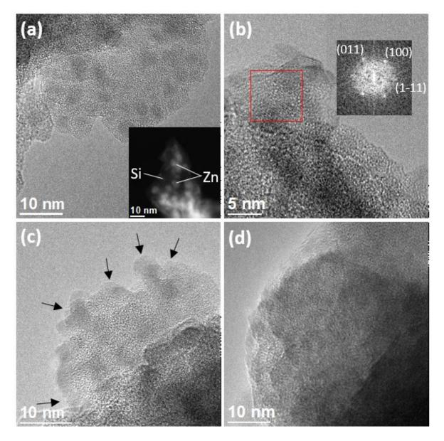
**Figure 4.5** TEM images of *x*Si-1A ZnO nanohybrids. (a) TEM and HAADF image (inset) of 3.8Si-1A. (b) HRTEM image of 3.8Si-1A with the inset showing fast Fourier transformed (FFT) image of the red square area. (c) HRTEM of 1.1Si-1A. (d) HRTEM of 10Si-1A.
