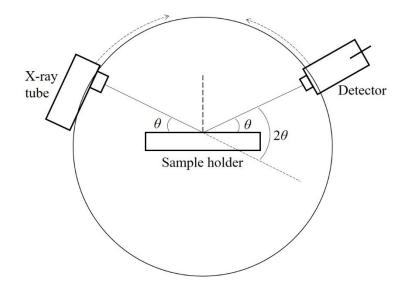
Figure 2.3 XRD setup for the study of polycrystalline materials.
