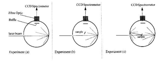
**Figure 2.12** Illustration of three configurations with an integrating sphere for PL QY measurement. (a) The sample is not present in the sphere. (b) The sample is present but the laser is not directed onto the sample. (c) The sample is present and the laser in directed onto the sample.
