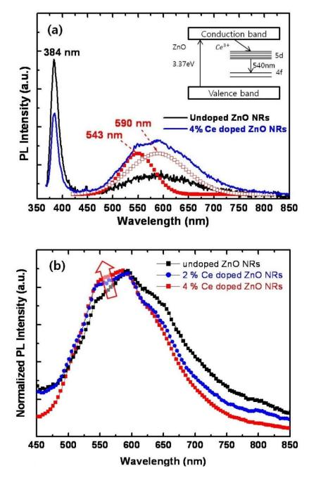
**Figure 1.13** (a) PL spectra of undoped ZnO and Ce-doped ZnO. The inset shows a schematic diagram of Ce<sup>3+</sup> electronic levels in ZnO bandgap. (b) Normalized PL spectra in the visible range of undoped and Ce-doped ZnO.
