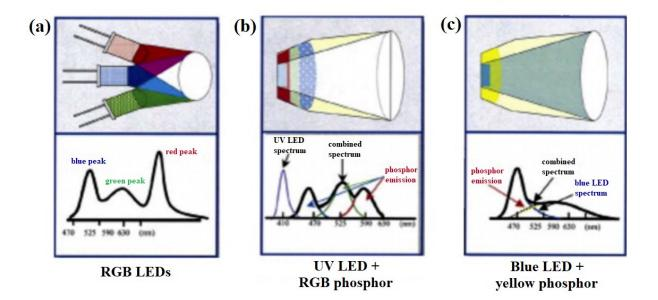
**Figure 1.1** Three approaches to generate white light with LEDs: (a) with single RGB LEDs, (b) with full conversion of UV LED, and (c) with partial conversion of blue LED. [7]
