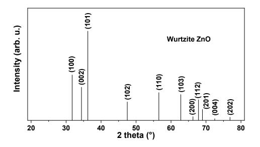
Figure 2.5 Theoretical diffraction lines of polycrystalline wurtzite ZnO.
