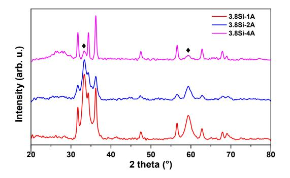
Figure 4.9 XRD spectra of 3.8Si-yA (y = 1, 2 and 4) ZnO/PAA nanohybrids.
