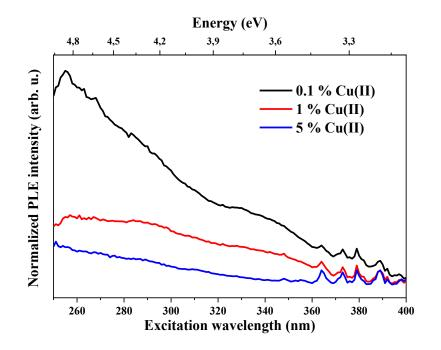
Figure 3.17 PLE spectra of Cu(II)-doped ZnO nanohybrids at three doping concentrations.
