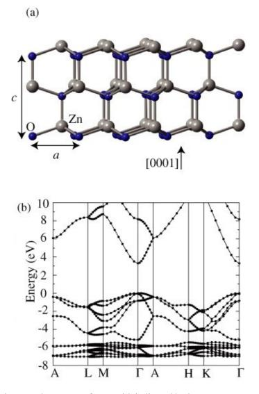
**Figure 1.5** (a) Wurtzite crystal structure of ZnO with indicated lattice parameters a and c. (b) Calculated band structure of ZnO. The energy of the valence band maximum was set to zero. [55]
