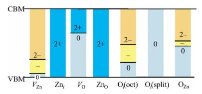
Figure 1.9 Thermodynamic transition levels for defects in ZnO. [78]
