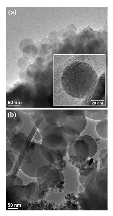
Figure 3.1 Morphologies of (a) 0.1 % Mn-doped ZnO nanohybrid and (b) 5 % Mn-doped ZnO nanohybrid.
