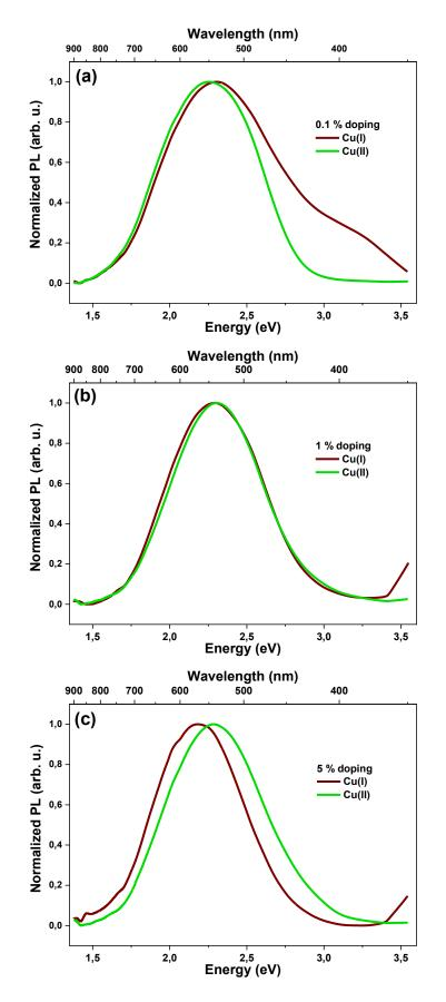
**Figure 3.14** PL spectra of Cu-doped ZnO nanohybrids with two different Cu valences (+1 and +2) at (a) 0.1 %, (b) 1 %, and (c) 5 % doping concentrations.
