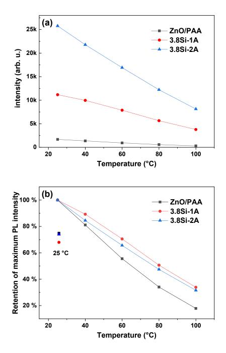
**Figure 4.19** Evolution of (a) maximum PL intensity and (b) retention of maximum PL intensity relative to the initial maximum at different temperatures up to 100 °C of uncoated ZnO/PAA, 3.8Si-1A, and 3.8Si-2A. The three points standing alone at 25 °C in (b) represent the retentions of maximum PL intensity after cooling down.
