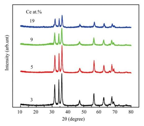
Figure 1.12 XRD patterns of Ce-doped ZnO nanoparticles. [110]
