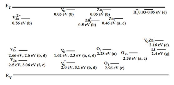
**Figure 1.10** Transition levels (measured with respect to the edge of the conduction band) of defects in ZnO reported in literature by different groups. (a) Ref [83]. (b) Ref [84]. (c) Ref [85]. (d) Ref [86]. (e) Ref [87]. (f) Ref [78]. (g) Ref [88], [89].
