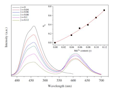
**Figure 1.3** PL spectra of Ba<sub>2</sub>Ca(B<sub>3</sub>O<sub>6</sub>)<sub>2</sub>:0.04Eu<sup>2+</sup>, yMn<sup>2+</sup> phosphors ( $\lambda_{ex} = 330$  nm). Inset shows the dependence of the energy transfer efficiency  $\eta_T$  on the Mn<sup>2+</sup> content (y). [18]
