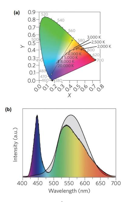
**Figure 1.2** (a) Commission Internationale de l'Éclairage (CIE, 1931) diagram with a black-body radiation curve (black solid line) and CCT values. (b) Luminescence spectrum of YAG:Ce and human eye sensitivity curve in grey-shaded spectrum. [7]
