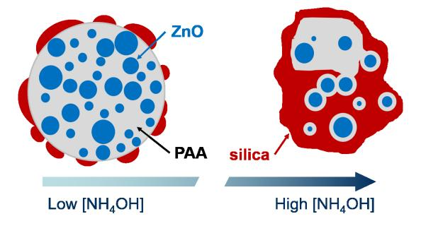
**Figure 4.14** Structure model of silica-coated ZnO/PAA nanohybrids under different concentrations of NH<sub>4</sub>OH in solution A.
