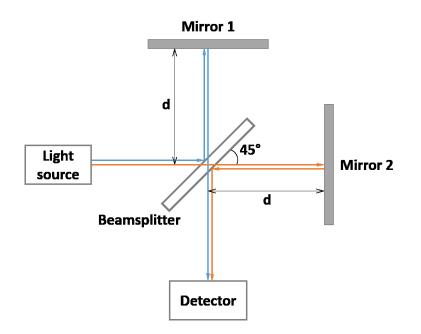
Figure 2.8 Schematic of a Michelson interferometer.
