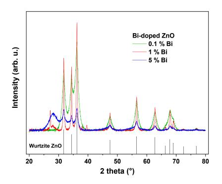
Figure 3.8 XRD spectra of Bi-doped ZnO nanohybrids.
