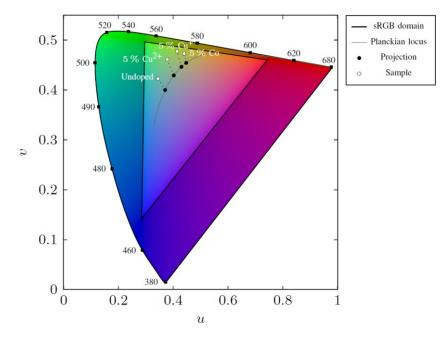
**Figure 3.19** Position of the spectra of selected doped samples in the gamut chart in Judd's UCS diagram (figure produced by Fabien Mandorlo).
