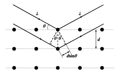
Figure 2.4 X-ray scattering from crystalline planes.
