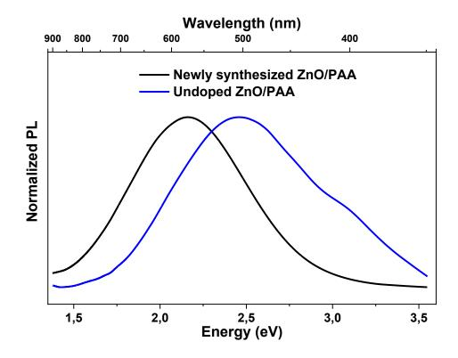
Figure 4.1 Normalized PL spectra of ZnO/PAA synthesized in two different batches.
