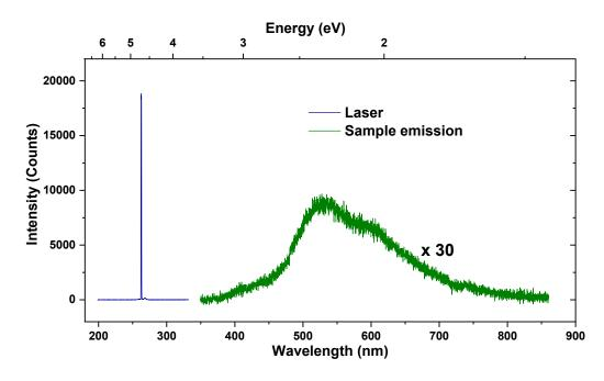
**Figure 2.15** Typical laser profile and emission profile from measurement (c) for ZnO nanohybrids. The emission profile is enlarged 30 times.
