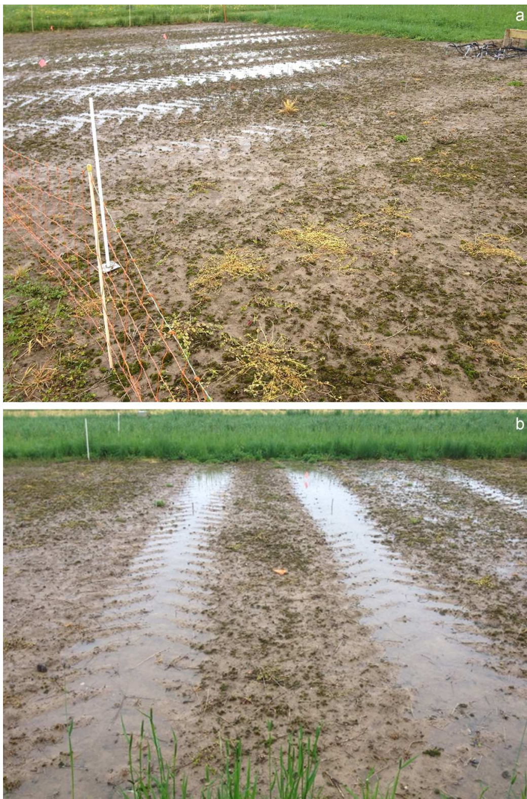
Fig. 8. Ponding water after rainfall in (a) compacted plots and (b) wheel tracks of the bare soil treatment in April 2015 (i.e., 1 yr after compaction).
