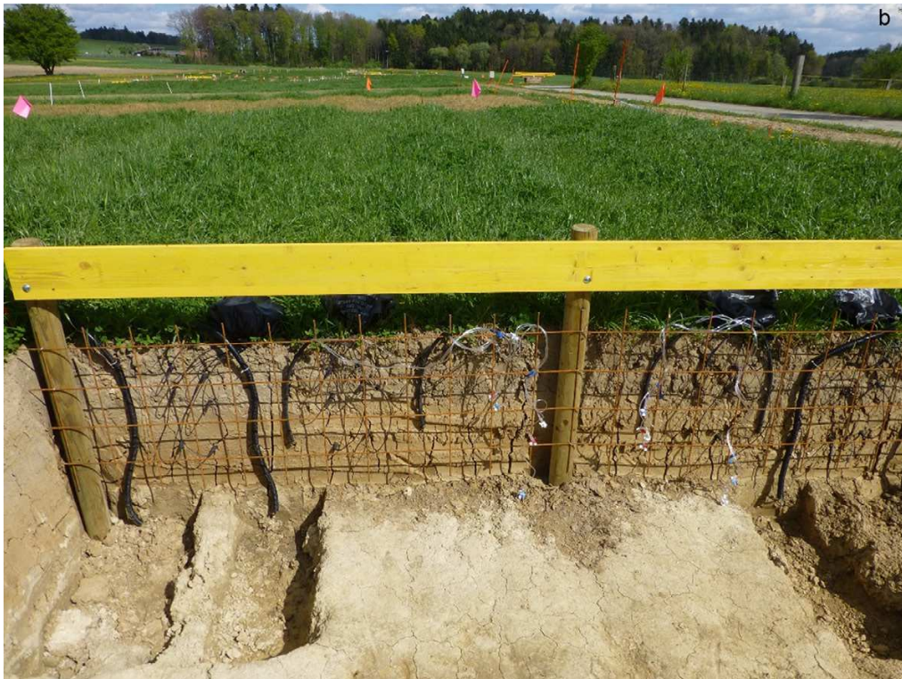
Fig. 3. (a) Schematic overview of a sensor bank, showing number and depths (0.1, 0.2, 0.4, 0.7, and 1.0 m) of the various sensor probes (but not necessarily the exact locations) installed from a profile wall at the plot edge through drilled holes of 0.6-m length; and (b) photo of a sensor bank where soil probes have been installed into the profile wall at various depths. The profile wall is at the plot edge.
