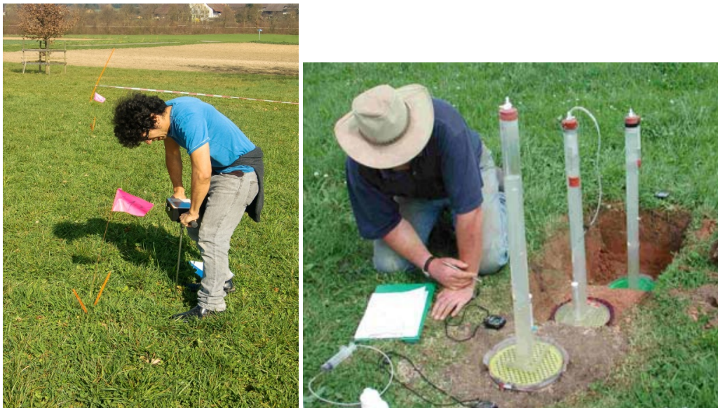
Figure 1.5 – Examples of in-situ measurements of soil properties. (a) Cone penetrometer test for measuring mechanical properties of soils. Photo from the experiment by Keller et al. (2017). (b) Disc permeameter for measuring surface infiltration and saturated hydraulic conductivity of soils. Credits to http://vro.agriculture.vic.gov.au .
