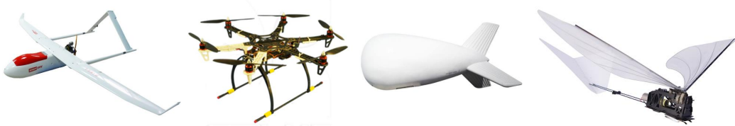
Figure 1.2: From the left to the right: fixed-wing, rotary-wing, blimp and flapping-wing airframes
