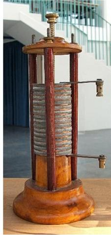
Figure I.2 Pile de Volta
