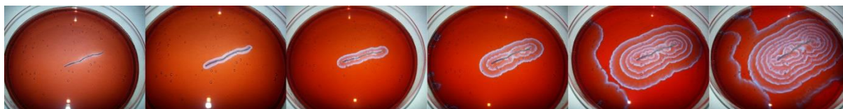
Figure 1.5. Patterns, produced by the B-Z reaction, starting from initially homogeneous solution in Petri dish after perturbation with silver thread. Figure was taken from https://debanupf.wordpress.com/author/debanupf/
