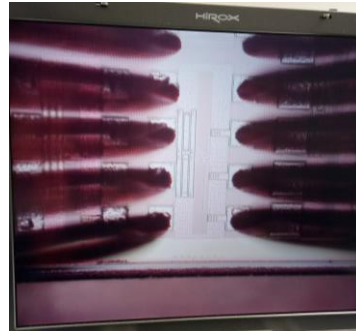
Biomimetic neuron under probes.
