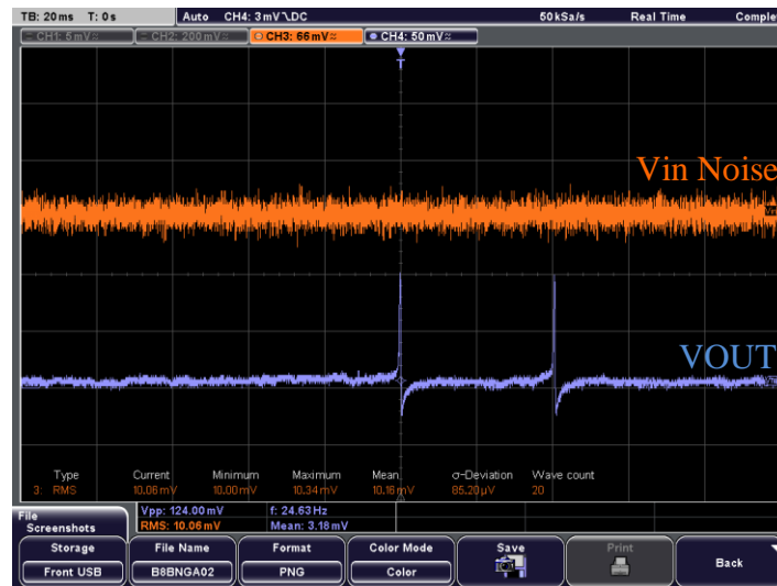
Figure 4.13 Response of biomimetic neuron to the low level of Gaussian noise.
