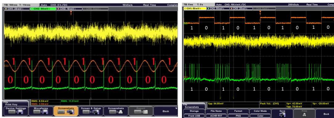
Figure 4.38 Detecting states: Left: sinusoidal signal detected using stochastic resonance phenomena with error. Right: square signal detected using stochastic resonance phenomena without error.
