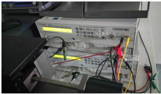
Two Agilent SMU (E5273A and E6263A) connected to VDD, VDD_T, VDDANA and ISSANA pads.
