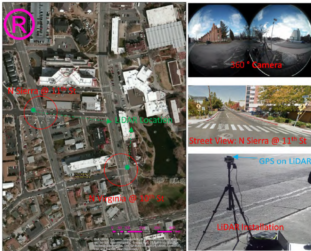
FIGURE 1.3: Vehicles' trajectories extraction using the 360-degree (rotating) LiDAR [2].
