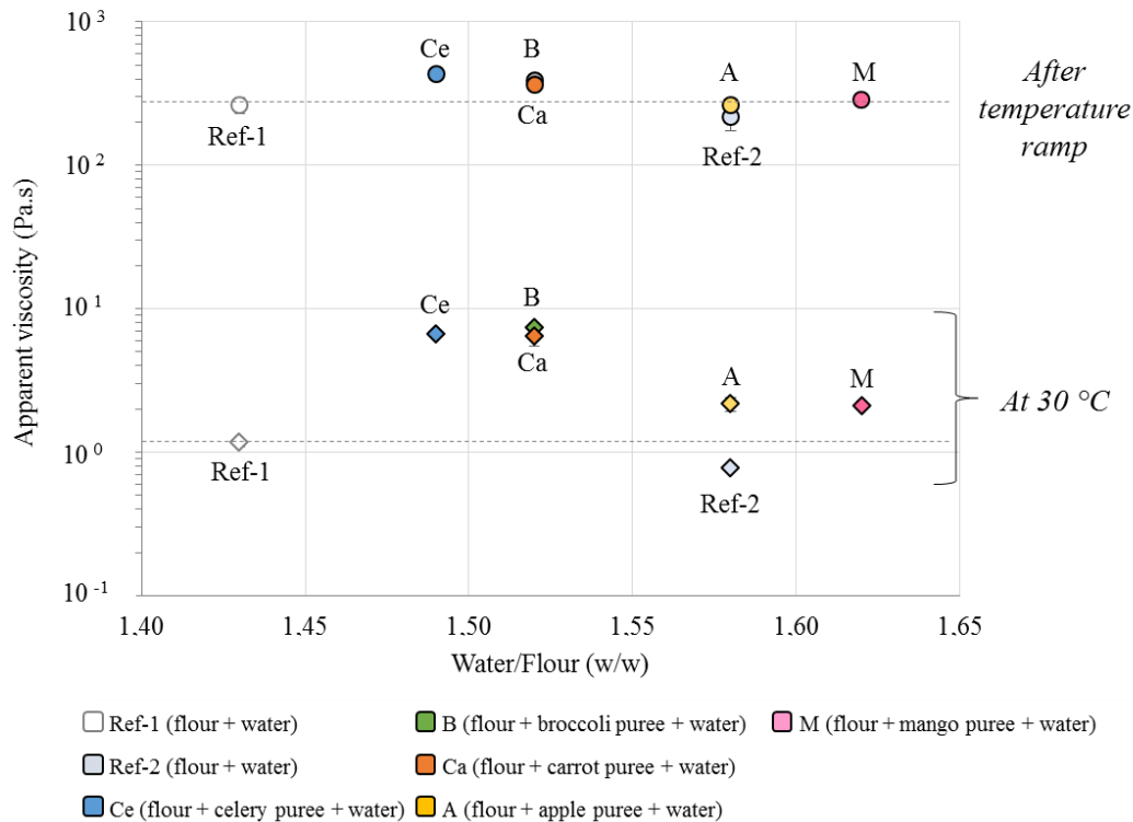
Fig. 14: Apparent viscosity values extracted from the viscosity temperature curves measured at 8 \text{ s}^{-1} , using the starch cell fitted on the MCR301 rheometer. Diamonds : viscosity measured at 30 \text{ }^\circ\text{C} . Circles : peak viscosity.
