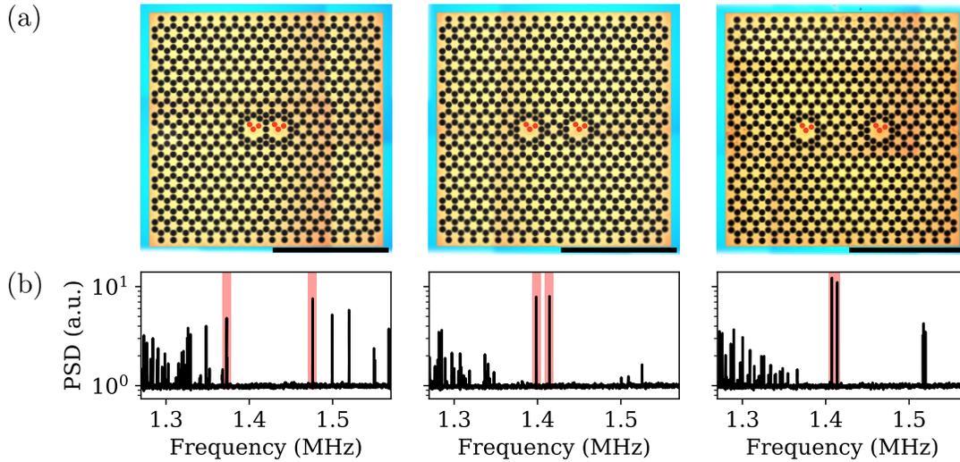
Figure 4.25: **a**, Optical micrographs of dimer membranes, for a dimer separation of 1, 3, and 5 unit cells (from left to right). The red points indicate the locations where the thermal spectra were measured. **b**, Measured compiled thermal spectra in the central defect area, for the membrane design which lies directly above them. The red area highlights the two D1 modes which become the D1<sup>+</sup> and D1<sup>-</sup> modes when hybridized.
