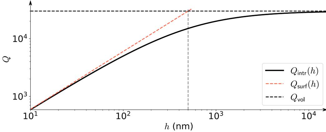
Figure 3.3: Variation of  $Q_{\text{intr}}$  with the thickness for SiN membranes. The gray dashed line represents the thickness for which surface and volume losses contribute equally to the  $Q_{\text{intr}}$ .
