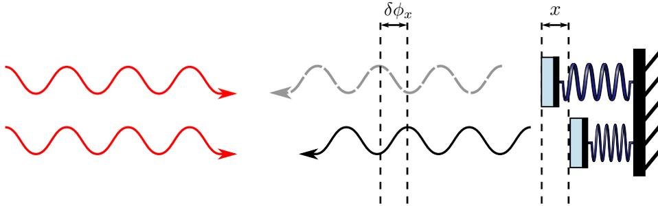
Figure 1.3: Schematic representation of the relative phase shift of a light beam due to the displacement of a reflective surface.
