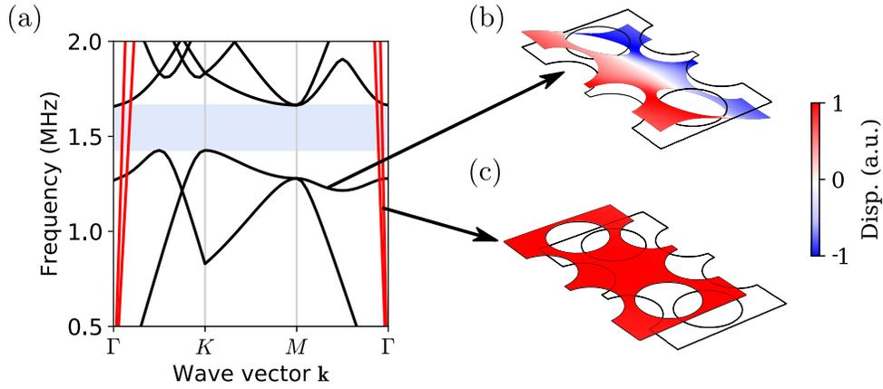
Figure 3.9: **a**, Simulated band diagram for a PnC with a hexagonal unit cell with  $b = 160 \mu\text{m}$ ,  $r = b/4 \mu\text{m}$ , and  $\sigma_0 = 1 \text{ GPa}$ . The modes highlighted in red are in-plane modes with high velocities. The area highlighted in blue is the inferred quasi-bandgap. **b-c**, Displacement (Disp.) profile of a single unit cell, for: **(b)** an out-of-plane crystal mode, and **(c)** an in-plane crystal mode. The unit cell at rest is shown as a black contour.
