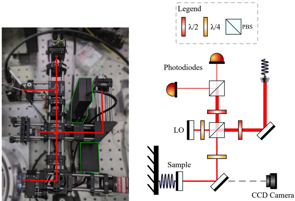
Figure 4.8: **(left)** Photograph of the monolithic interferometer. The beam path is drawn in red, and the visible parts of the translation stages are contoured in green. **(right)** Schematic representation of the interferometer shown left. Lenses have been omitted for clarity. Although this setup looks very similar to a Michelson interferometer, it can be shown to be formally equivalent to a Mach-Zehnder due to the  $\lambda/4$  plates in front of the sample and the LO.
