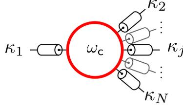
Figure 1.7: Illustration of a resonator of frequency  $\omega_c$ , coupled to  $N$  ports, with a coupling  $\kappa_j$  to the  $j^{\text{th}}$  port. In most models, one or two ports are chosen as the input/output ports, and all others are grouped together as a single effective port through which information is irreversibly lost.
