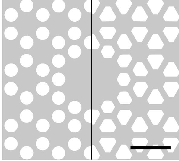
Figure 5.1: **(left)** Current design of the PnC membrane. **(right)** Optimized PnC membrane design, tweaking the shape of the central defect and of the PnC holes to optimize the mode profile. SiN is shown in gray, and the scale bar represents  $200 \mu\text{m}$ . The author thanks L. Najera for his help with this figure.
