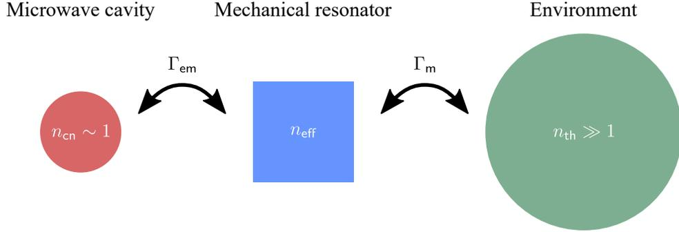
Figure 1.12: Illustration of the mechanical resonator (shown as a square), of population  $n_{eff}$ , in an electromechanical cooling experiment. It is coupled to two baths (shown as circles): the thermal environment, with a population  $n_{th} \gg 1$ , at a rate  $\Gamma_m$ , and to the microwave resonator, with an effective population  $n_{cn} \sim 1$  (derived below), at a rate  $\Gamma_{em}$ .
