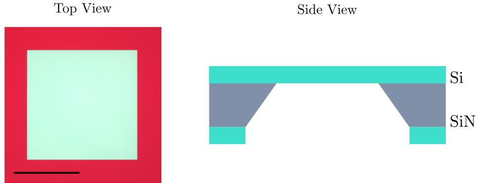
Figure 2.2: **(left)** Optical micrograph of a SiN membrane fabricated by the optomechanics group of the LKB. Suspended SiN is seen in light blue, and SiN above Si is seen in magenta. The membrane has a thickness of 200 nm. The black scale bar represents 0.5 mm. **(right)** Side view of the mechanical resonator, not to scale. The Si substrate is about 500- $\mu\text{m}$  thick, whereas the SiN thickness is approximately 100 nm.
