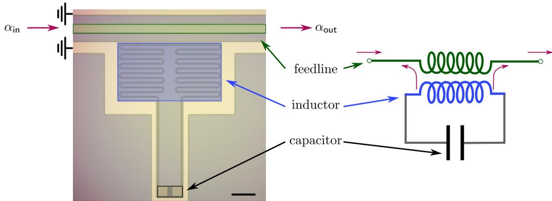
Figure 2.4: **(left)** Optical micrograph of a lumped-element microwave cavity, from the sample labelled BM2. Nb is shown in yellow, and the Si substrate in gray. The feedline is highlighted in green, the inductance in blue, and the capacitor pads in black. The scale bar represents  $150 \mu\text{m}$ . **(right)** Equivalent circuit to the cavity, with the circuit elements colored following the same code as in the image.
