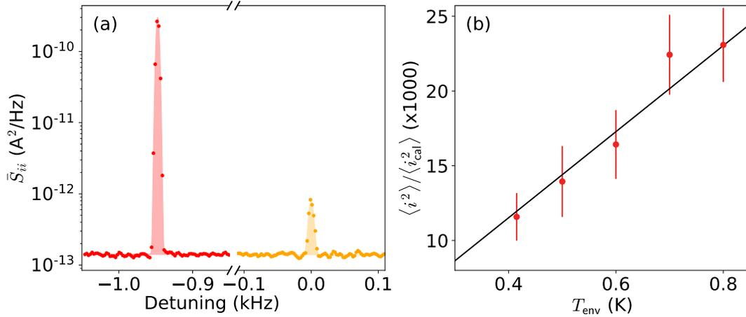
Figure 2.8: **a**, Calibration (red) and mechanical (yellow) sidebands of the probe. The filled areas are Gaussian fits. **b**, Repetition of the spectrum acquisition of **(a)** for various cryostat temperatures. The solid black line is a linear fit.
