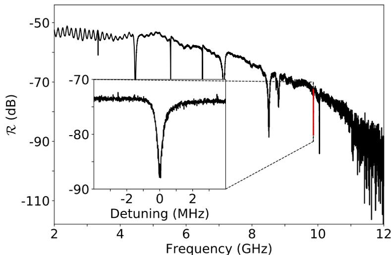
Figure 2.6: Reflection spectrum  $\mathcal{R}$  of the sample labeled BM2. Several resonance peaks are present, with the cavity resonance highlighted in red. Inset is a close-up on the cavity resonance.
