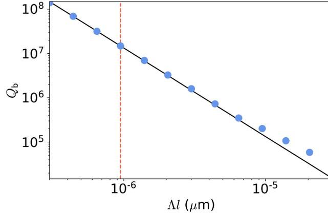
Figure 3.14: Variation of  $Q_b$  with the dissipation dilution factor  $\Lambda l$ , for D1. The simulation was run by varying  $\sigma_0$ , keeping all other parameters. The blue points are the simulated data while the black line represents a fit with  $1/\Lambda^2$ . The dashed red line represents typical sample parameters.
