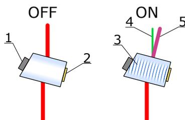
Figure 4.13: Principle of the AOM. The incident beam is shown in red 1: mechanical absorber. 2: Piezoelectric actuator. 3: Acoustic wave. 4: 0<sup>th</sup> order beam (green). 5: 1<sup>st</sup> order beam (violet). ©By Wikimedia Commons User:Ximeg / CC BY-SA 3.0
