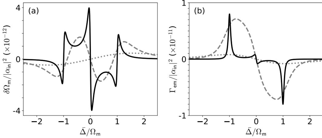
Figure 1.11: **a-b**, Shift in **(a)** the mechanical resonance frequency and **(b)** the electromechanical damping rate, for various pumping frequencies  $\bar{\Delta}$ . For both figures, various values of  $\kappa/\Omega_m$  are taken, namely: 0.1 (black), 1 (gray, dashed) and 4 (gray, dotted). The black curve is representative of the electromechanical device parameters presented in chapter 2, with typical values  $g_0 = 1$  Hz,  $\Omega_m = 500$  kHz, and  $\eta = 1/2$ .
