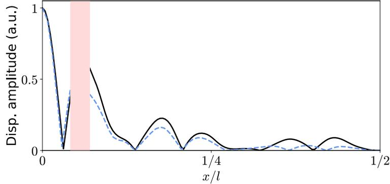
Figure 3.12: Displacement (Disp.) amplitude of D1 for  $\Lambda l \approx 30 \mu\text{m}$  (black) and for  $\Lambda l \approx 1 \mu\text{m}$  (blue, dashed). For these plots, all parameters were kept fixed except for  $\sigma_0$ , which was taken as 1 MPa and 1 GPa, respectively. The red region represents a hole in which no data can be acquired.
