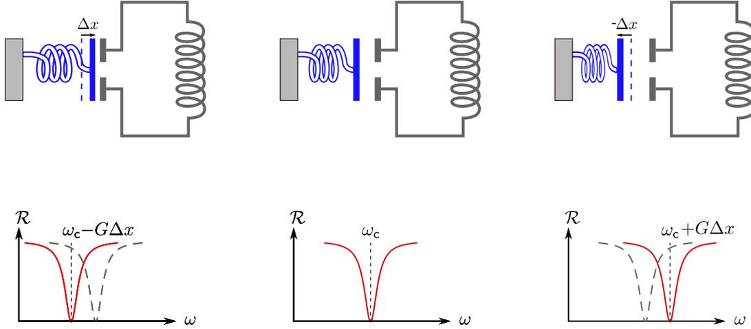
Figure 1.10: **(Center)** Illustration of a dispersively coupled electromechanical system with a mechanically compliant capacitor. Below, the typical reflection of the circuit is shown. If the mobile capacitor plate moves closer to **(left)** or farther away from **(right)** the static capacitor plate by a small distance  $\Delta x$ , the frequency of the circuit decreases or increases by  $G\Delta x$ . The drawing is not to scale.
