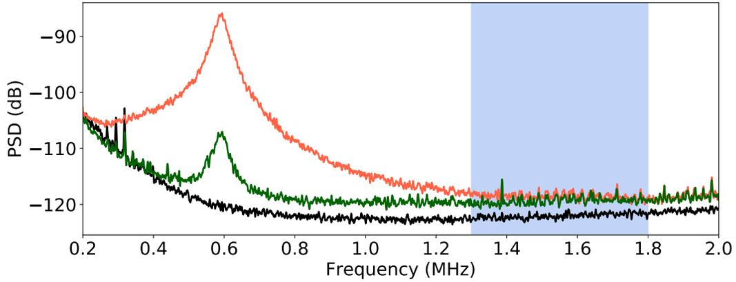
Figure 4.11: PSD of the interferometer when the balancing is poorly optimized (red), and when  $\beta_{\Delta}$  is minimized (green). In addition, we show the electronic noise floor of the setup, measured with the laser turned off (black). The blue area indicates the frequency range of interest for characterizing the PnC membranes presented in this work. Here,  $P_0 = 30$  mW.
