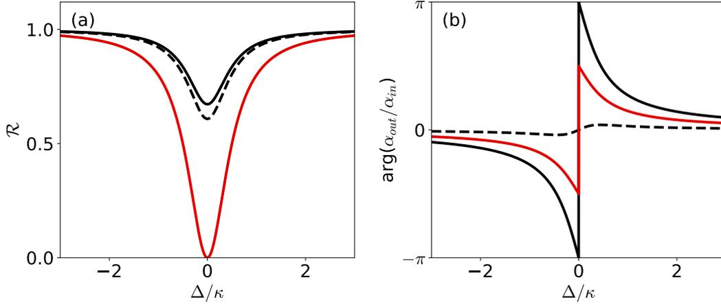
Figure 1.9: **a-b**, The response of a bare harmonic circuit in the reflection configuration, for fixed  $\kappa$ . The reflection coefficient is shown in **(a)**, and the phase of the reflected signal is shown in **(b)**. Three different cases are considered:  $\eta = 0.91$ , the undercoupled case depicted by the dashed black line,  $\eta = 0.11$ , the overcoupled case depicted by the solid black line, and  $\eta = 0.5$ , the critically coupled case depicted by the solid red line.
