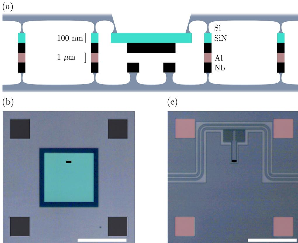
Figure 2.5: **a**, Schematic representation of the electromechanical device, seen through a cut plane normal to the surface. The diagram is not to scale, and the ground planes have been omitted for clarity. **b-c**, Optical micrographs of a metalized SiN membrane (**b**) and the LC cavity circuit (**c**) from the sample labeled BM2. The relevant areas have been colored to correspond to the material color-coding set by (**a**). The white scale bars represent 1 mm.
