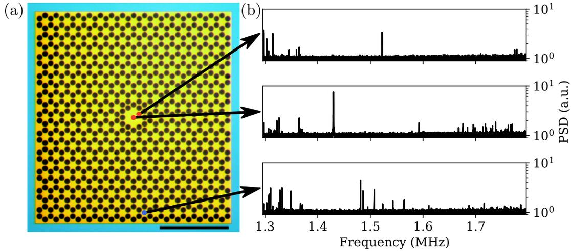
Figure 4.15: **a**, Optical micrograph of a PnC membrane of a generation 1 design. In yellow, the SiN is freely standing, and in light blue it is lying above Si. The points indicate the positions at which the spectra of **(b)** are measured. **b**, Three different spectra of the mechanical motion, taken at various points on the membrane.
