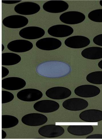
Figure 5.2: Scanning electron microscope image of a metalized PnC membrane. SiN is shown in dark yellow, and Nb is shown in blue. The scale bar represents  $300 \mu\text{m}$ . Image courtesy of T. Capelle [43].
