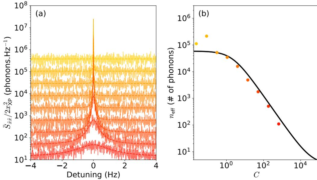
Figure 2.10: **a**, Phonon noise spectra in an electromechanical cooling experiment. The centers of the peaks are shifted to be centered around 0. The full lines represent experimental data and the dashed lines are Lorentzian fits to the peaks. From orange to red we show the spectra for increasing cooperativities  $C$ , following the colors of the data points in **(b)**. **b**, The data points represent the extracted phonon population. The full line represents a fit to the data of eq. (2.6).
