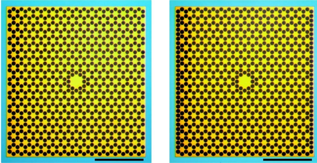
Figure 4.5: Optical micrographs of fabricated SiN membranes, structured with a hexagonal lattice PnC. **(Left)** The membrane has no additional patterning on its vertical edges, contrary to **(Right)**, where a series of holes is added.
