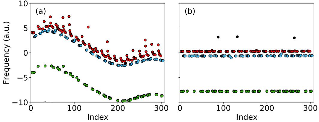
Figure 4.17: **a**, Frequency of three modes near 1.4 MHz as a function of the laser position index. Three modes were identified “by eye”, and shown in red, green, and blue. **b**, Corrected frequency of the modes shown in (a). The laser position dependence of the frequency is removed by dividing by the frequency of the fundamental mode, shown in fig. 4.16b.
