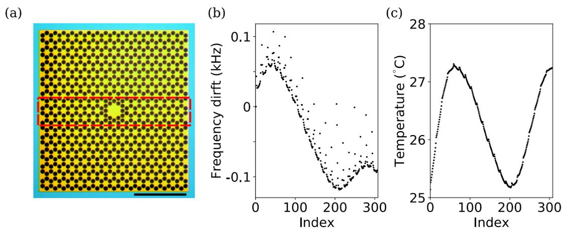
Figure 4.16: **a**, Optical micrograph of a generation 1 membrane, highlighting by the red rectangle the area over which the raster scan discussed in this section is performed. **b**, Frequency of the fundamental mode of a PnC membrane, at approximately 209 kHz, as a function of the laser position index. **c**, Temperature of the sample holder over the course of a scan.
