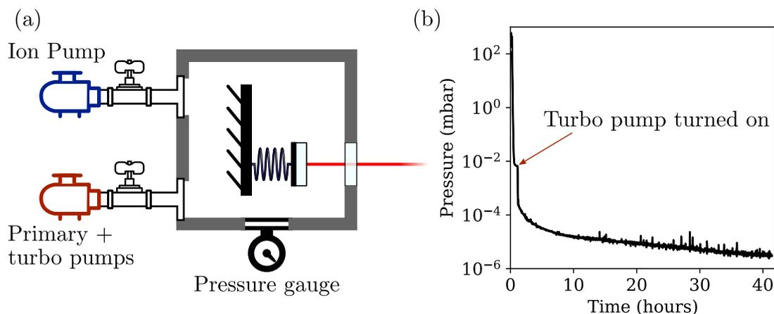
Figure 4.7: **a**, Schematic representation of the vacuum system, pumped in parallel by a primary and turbomolecular (turbo) pump bank, and an ion pump. The red beam indicates the optical access of the chamber to the sample. *Pump icon made by Freepik from www.flaticon.com.* **b**, Pressure evolution in a typical pumping cycle using only the primary and turbo pumps.
