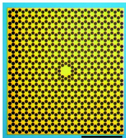
**Figure 1- Optical micrograph of a patterned SiN membrane.**
