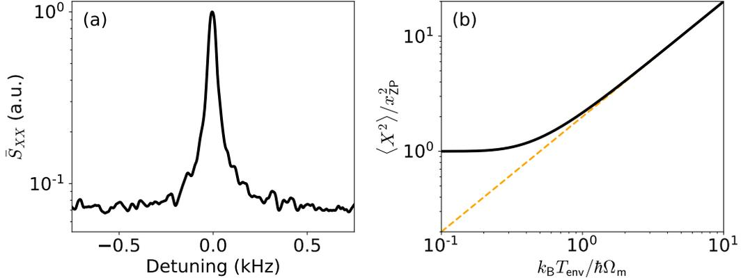
Figure 1.2: **a**, Experimentally measured noise spectrum of the position of a mechanical mode, with a central frequency of 1.47 MHz. The spectrum is plotted against the detuning from the center of the peak. Away from the Lorentzian, the noise floor does not reach zero as additional sources of noise are usually present in a measurement. **b**, Quantum (black) and classical (dashed orange) dependencies of the variance of  $x$  with the temperature.
