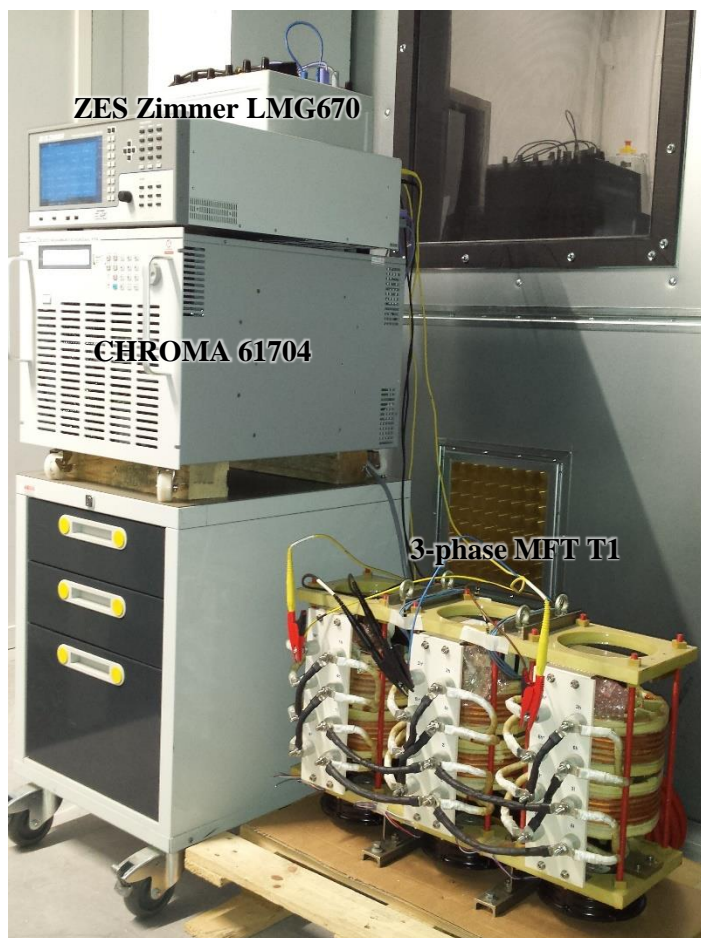
Fig. A14. MFT T1 no load test with a variable frequency 3-phase sinusoidal power supply
