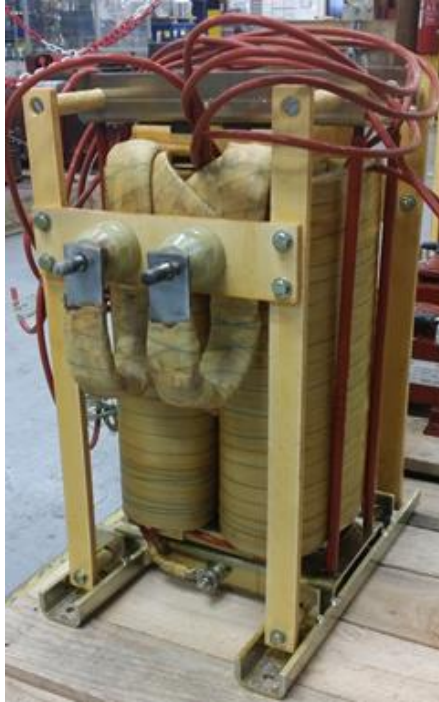
Fig. A1. Single-phase MFT prototype 180 kVA [139]
