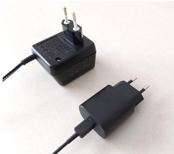
Fig. 2.19. Illustrative comparison between a 50 Hz transformer-rectifier (top left) and a solid-state transformer (bottom right)
