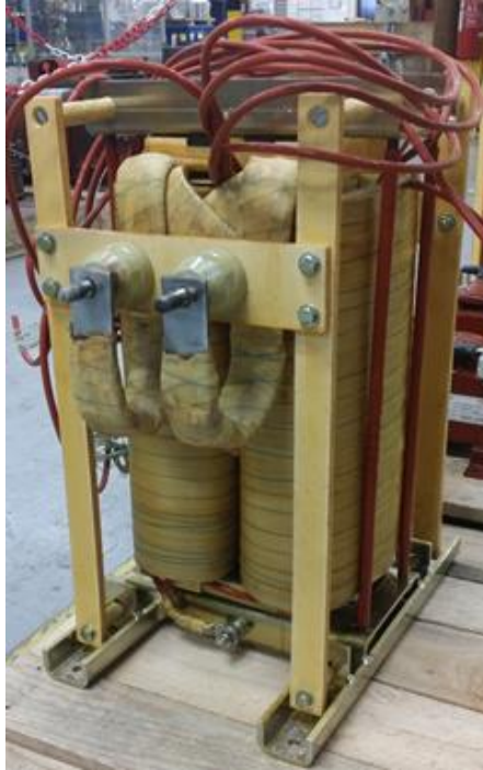
Fig. A1. Single-phase MFT prototype 180 kVA [139]
