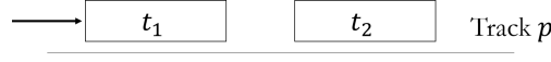
Figure 4.4: An intermediate train t_1 enters a track p through the left side after an intermediate train t_2 . Then t_1 is placed on the left side of t_2 .
