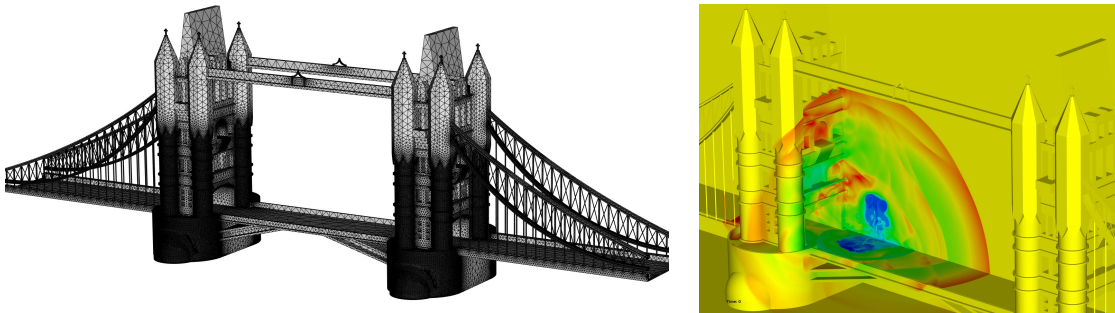
Figure 3.20 – Tower-bridge test case. Initial mesh and geometry (left) and density iso-values of the blast on an adapted mesh (right).
