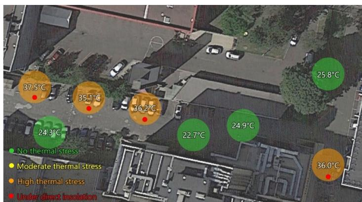
Figure 5: Thermal stress indicator (UTCI) on site before conversion measured on eight different locations on June the 26<sup>th</sup> of 2018, from 1 pm to 3 pm (local time)
