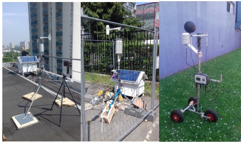
Figure 3: Rooftop (left) and parking lot (center) fixed and mobile (right) weather stations (before conversion).
