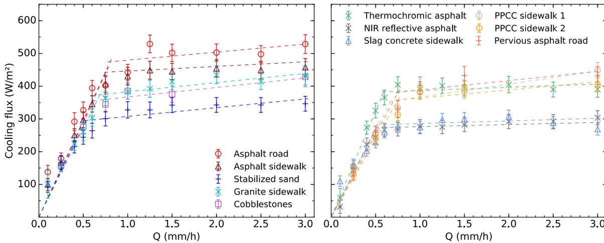
**Figure 18.3:** Total cooling flux  $\Phi$  as a function of the watering rate  $Q$  for traditional (left) and alternative pavements (right). The double piecewise linear regression is represented with dashed lines. (see Table 18.2) (Parison et al., 2020c).
