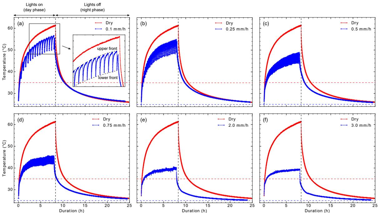
**Figure 12.1:** Asphalt road surface temperature with (blue) and without (red) watering for various watering rates (namely 0.1 (a), 0.25 (b), 0.5 (c), 0.75 (d), 2.0 (e) and 3.0 (f) mm/h). Horizontal dashed lines represent day (red) and night (blue) phases air temperature, while the black vertical dashed line marks the transition between day and night phases (Parison et al., 2020b).
