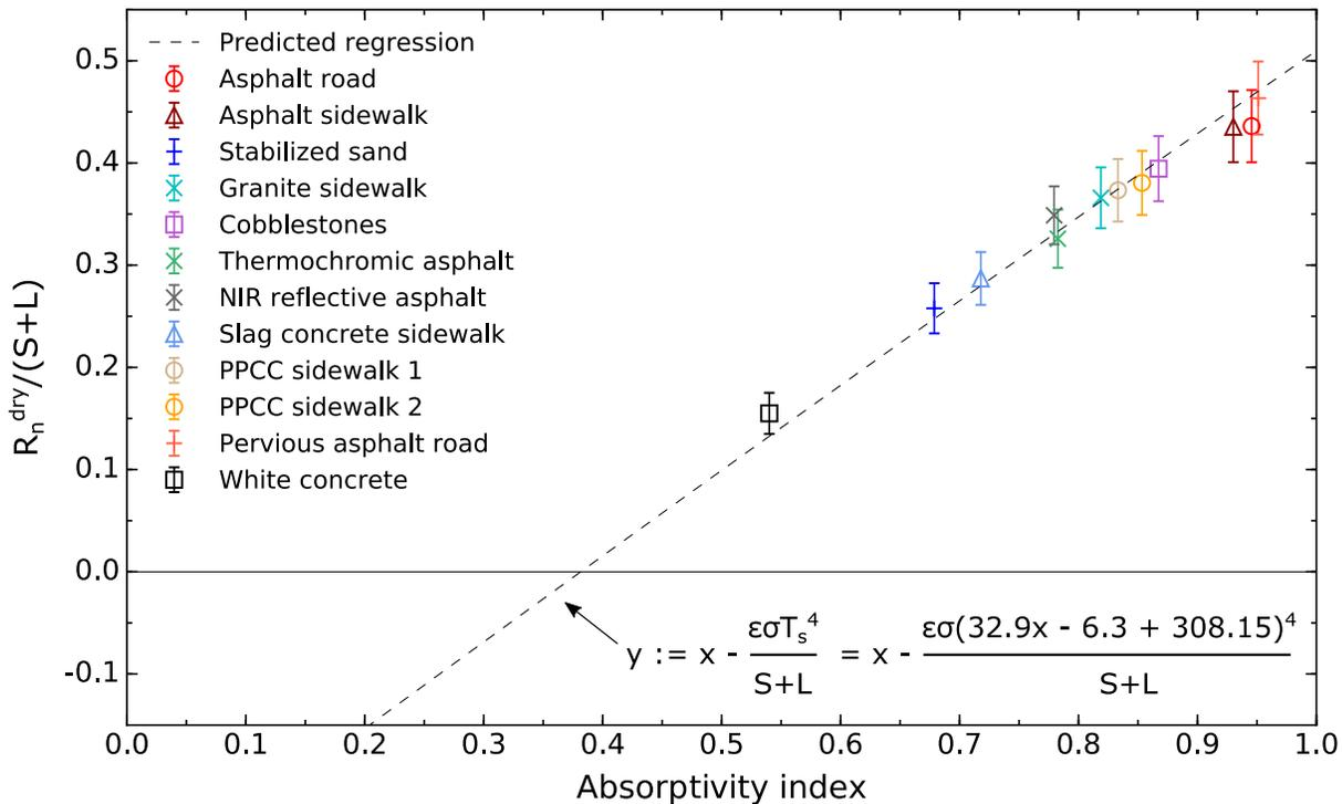
**Figure 23.1:** Steady-state net radiation to irradiance as a function of the absorptivity for non-watered pavements. The predictive behaviour (dashed) is obtained by injecting the linear regression of the surface temperature increase versus the absorptivity (Figure 17.2) into the analytical expression of  $R_n/S+L$ , as detailed on the Figure.
