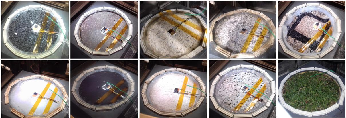
**Figure 16.2:** Photograph of some of the tested samples. From left to right and top to bottom: asphalt road, asphalt sidewalk, stabilized sand, granite sidewalk, cobblestones, thermochromic paint (>29°C), NIR reflective paint, slag concrete, PPCC sidewalk 1 and grass (Parison et al., 2020c).
