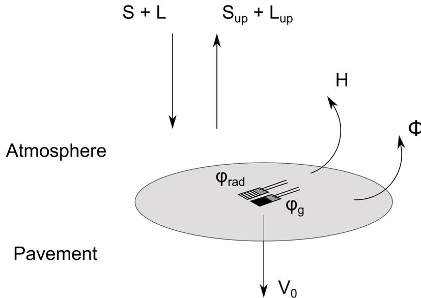
**Figure 11.5:** Schematic diagram of heat balance at the pavement surface.  $\phi_{rad}$  is the radiative flux measured by a radiative heat flow sensor and  $\phi_g$  the global heat flux measured by the fluxmeter (both sensors with  $\epsilon = 0.95$  and  $\alpha = 0.05$ ) (Parison et al., 2020c).
