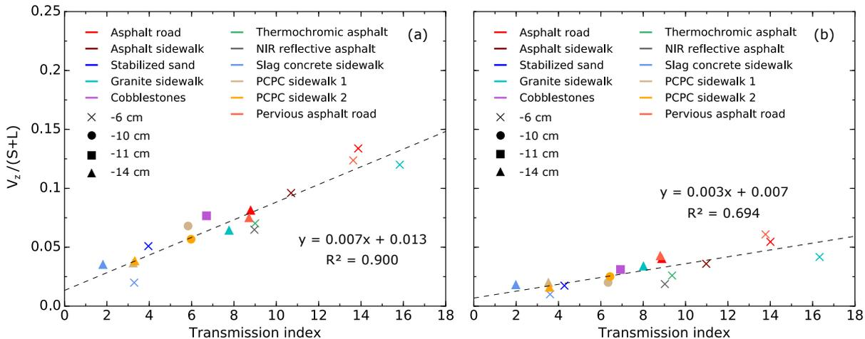
**Figure 19.3:** Steady-state heat fluxes in-depth (at 6, 10, 11 and 14 cm deep) to irradiance as a function of the transmission index for all pavements during a dry trial (a) and an optimally-watered trial (b) ([Parison et al., 2020c](#)).
