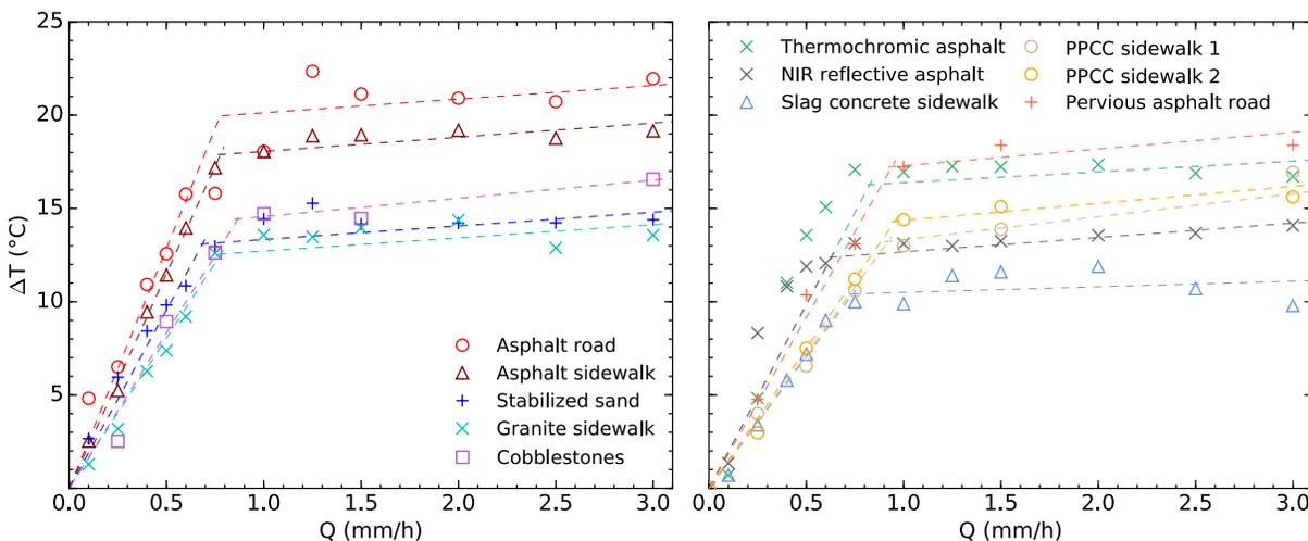
**Figure 18.1:** Maximum surface temperature dry-wet difference versus watering rate  $Q$  for traditional (left) and innovative pavements (right). The double piecewise linear regression is represented with dashed lines (see Table 18.1) (Parison et al., 2020c).
