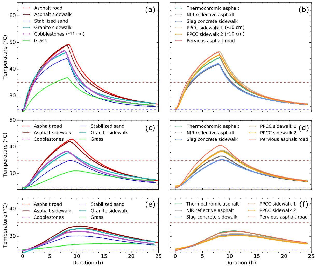
**Figure 17.3:** In-depth temperatures of standard (left-hand side) and innovative (right-hand side) dry pavement structures 6 (a and b), 14 (c and d) and 25 (e and f) cm deep. Dashed red and blue lines respectively represent day phase (35°C) and night phase (25°C) air temperature setpoints (Parison et al., 2020c).
