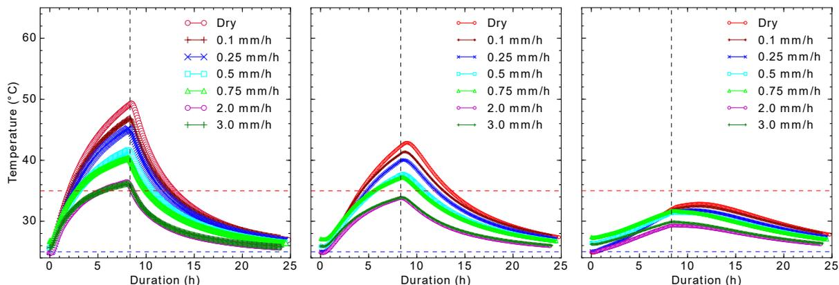
**Figure 12.4:** Asphalt road temperature 6 cm (left), 14 cm (center) and 25 cm (right) deep for non-watered and watered trials (i.e. 0.1, 0.25, 0.5, 0.75, 2.0 and 3.0 mm/h) (Parison et al., 2020b).
