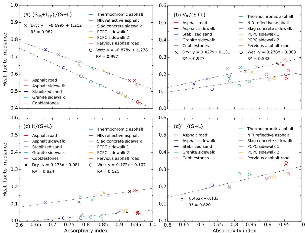
**Figure 19.1:** Steady-state surface partitioning of irradiance: (a): radiosity  $S_{up}+L_{up}$ , (b): conduction heat flux  $V_0$ , (c): atmospheric convective heat flux  $H$  and (d): cooling flux  $\Phi$ , all divided by irradiance  $S+L$  and plotted as a function of the absorptivity index  $a$  for all pavements. Non-watered trials are represented with cross markers while optimally-watered trials with circle markers (Parison et al., 2020c).
