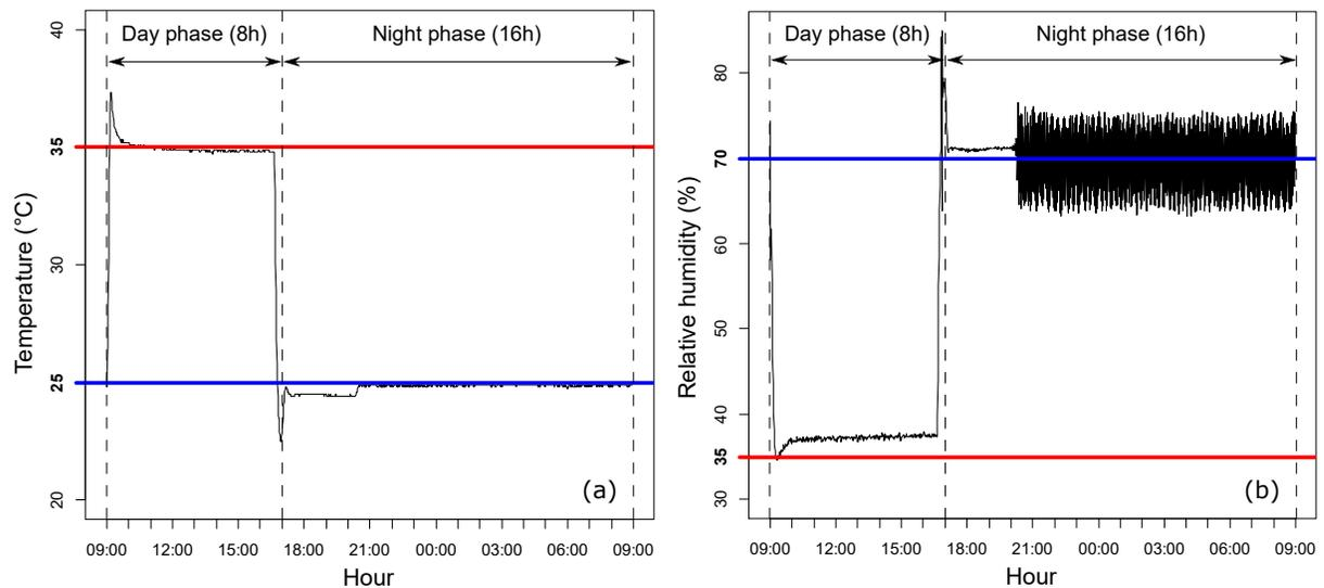
**Figure 11.2:** Temperature and relative humidity regulation over 24 h inside the climate chamber. Daytime and nighttime setpoints are indicated with horizontal red and blue lines, respectively (Hendel et al., 2018).
