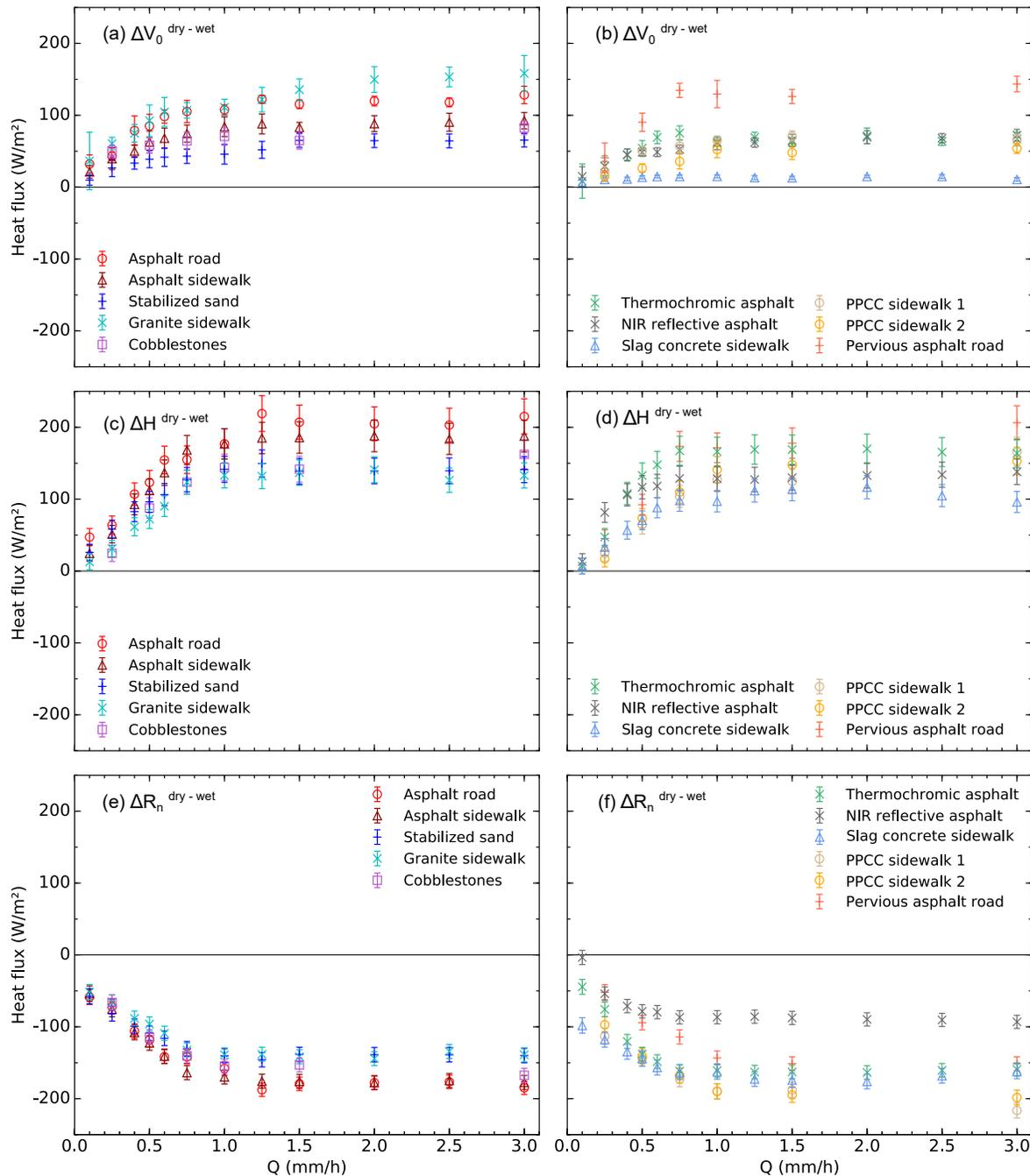
**Figure 18.2:** From top to bottom, dry-wet differences of conductive heat flux  $\Delta V_0^{dry-wet}$ , net radiation  $\Delta R_n^{dry-wet}$  and convective flux  $\Delta H^{dry-wet}$ , versus watering rate  $Q$ , for standard (left column) and innovative pavements (right column) (Parison et al., 2020c).
