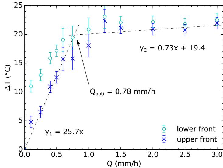
**Figure 12.3:** Dry-wet maximum surface temperature difference  $\Delta T_{max}^{dry-wet}$  for lower and upper fronts as a function of the watering rate for the asphalt road. A double linear piecewise regression with zero-intercept is used (dashed lines) to distinguish the two regimes (Parison et al., 2020b).
