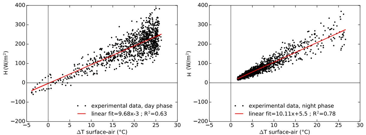
**Figure 12.8:** Asphalt road convective heat flux during the day phase (left) and the night phase (right) versus surface-air temperature difference, both fitted using a linear regression ([Parison et al., 2020b](#)).
