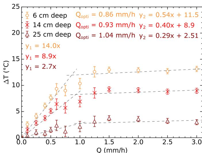
**Figure 12.5:** In-depth dry-wet maximum temperature difference  $\Delta T_{max}^{dry-wet}$  6 cm, 14 cm and 25 cm deep as a function of the watering rate for the asphalt road. Best double piecewise fits for both regimes and each depth are illustrated with dashed lines (Parison et al., 2020b).
