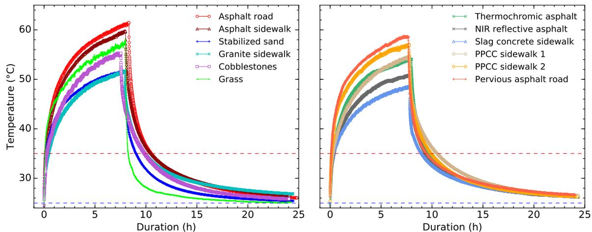
**Figure 17.1:** Surface temperatures of standard (left) and innovative (right) pavement structures over a 24-h non-watered trial. Dashed red and blue lines respectively represent day phase (35°C) and night phase (25°C) air temperature setpoints (Parison et al., 2020c).
