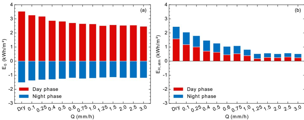
**Figure 12.9:** Stored (day phase) and released (night phase) pavement surface conduction energy density,  $E_0$  (a), and released (day and night phases) atmospheric convective energy density,  $E_{H,atm}$  (b), to watering rate (Parison et al., 2020b).
