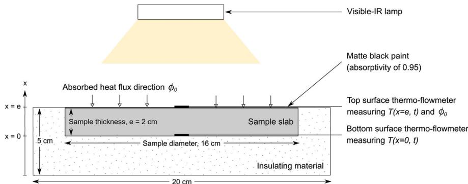
Figure 1. Diagram of the experimental set up.
