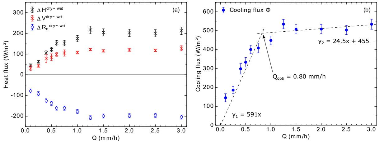
**Figure 12.10:** Dry-wet differences in net radiation  $\Delta R_n^{dry-wet}$ , in absorbed surface heat flux  $\Delta V_0^{dry-wet}$  and in atmospheric convective heat flux  $\Delta H^{dry-wet}$  (a), and total pavement cooling flux  $\Phi$  (b) to watering rate  $Q$  at the end of day phase. A double linear piecewise regression with zero-intercept is used on  $\Phi$  (b) (dashed lines) (Parison et al., 2020b).
