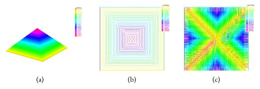
Figure 3.1: Left to right: 3D plot of the solution u, contour plot of u, the flux  $\phi$
