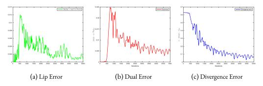
Figure 4.10: Error criterion for 5000 iterations and  $\tau=0.001$  and  $\eta=8/\tau$
