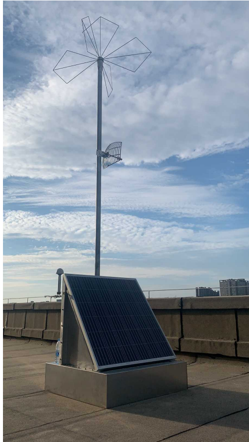
Figure 2.10: Picture of the HORIZONANTENNA detection unit, taken at Xi'an University. The bow-tie antenna design of the HORIZONANTENNA is placed on top of a 4 m long pole. At the bottom of the pole, the solar panel covers a triangular box where the electronics are stored. In the middle of the pole a WiFi antenna is placed for the data transfert. Credit: Zhang PengFei.
