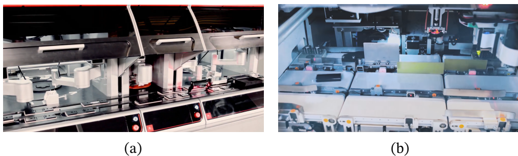
Figure 1.30: LFDA Xanthia modular microfactory [Gin20]. (a) Microfactory modules with robot arms manipulators and a frontal conveyor common to all modules. (b) Multi conveyors inside larger modules.
