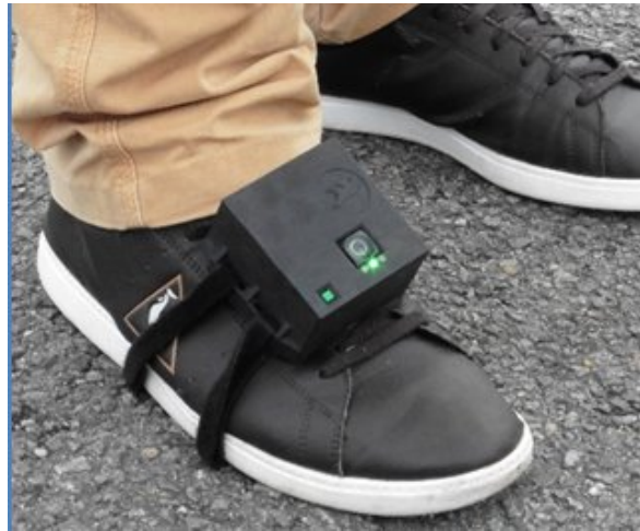
FIGURE 3.7 – Boîtier d'acquisition PERSY
