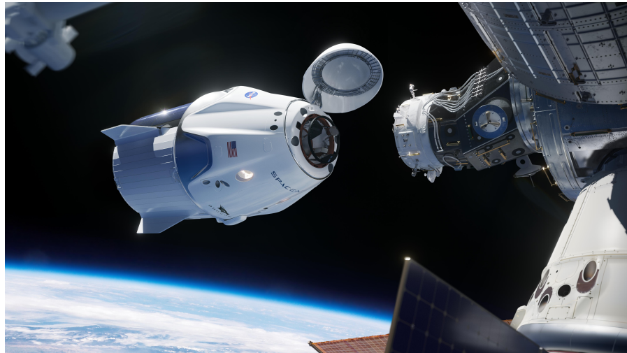
Figure 1.5: A SpaceX Dragon performing a docking manoeuvre with the ISS (Copyright free picture from NASA)
