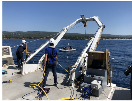
(b) The tether is managed manually by a crew member
