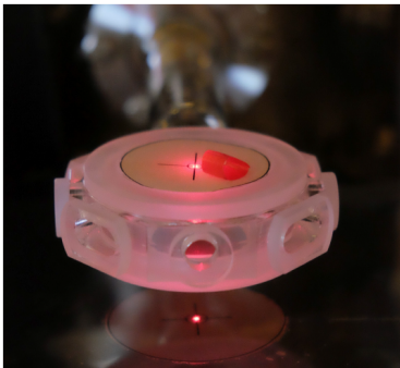
Figure 5.4. – The science cell during installation (Figure adapted from [135]). Its octagonal shape gives optical access from eight directions. The windows are coated and slightly tilted with respect to each other to minimize reflections. The top and bottom windows are recessed to allow the imaging optics to come as close as possible to the atomic sample. Here, a paper sheet has been put on top of the cell to align a pilot beam for the microscope alignment.
