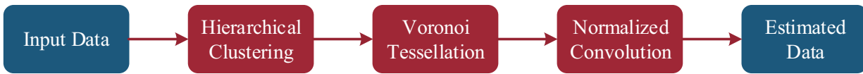
Figure 6.5: Sketch of the main steps of the methodology based on Voronoi tessellation and hierarchical clustering.
