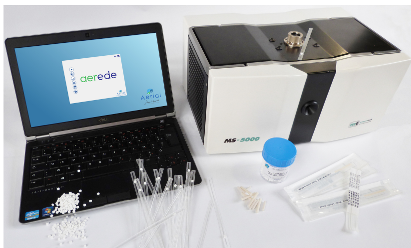
FIGURE 5.6: Aer'EDE2019 software and the MS5000 EPR spectrometer used for alanine dosimeters readout.
