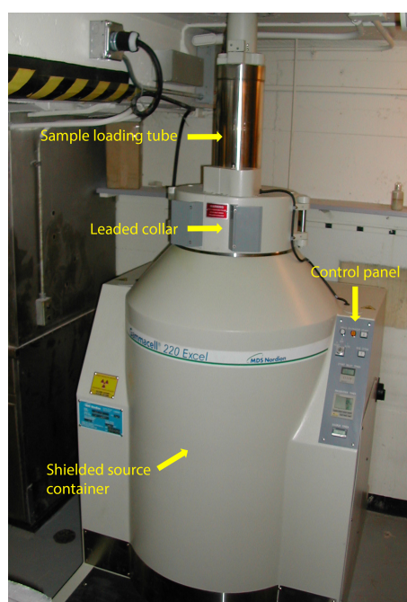
FIGURE 2.3: Gammacell200 ® , a self-shielded gamma irradiator.
