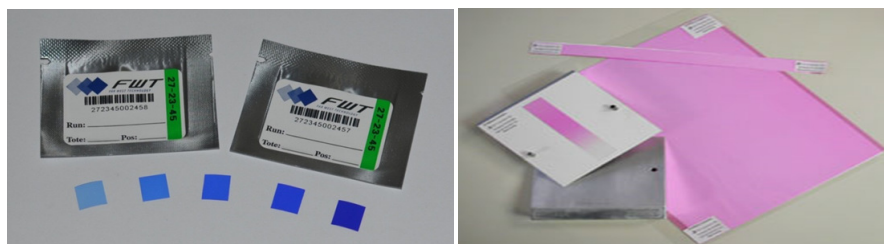
FIGURE 3.7: Two radiochromic dye films used as routine dosimeters in radiation processing: FWT-60 (blue) and B3-Risø (pink).
