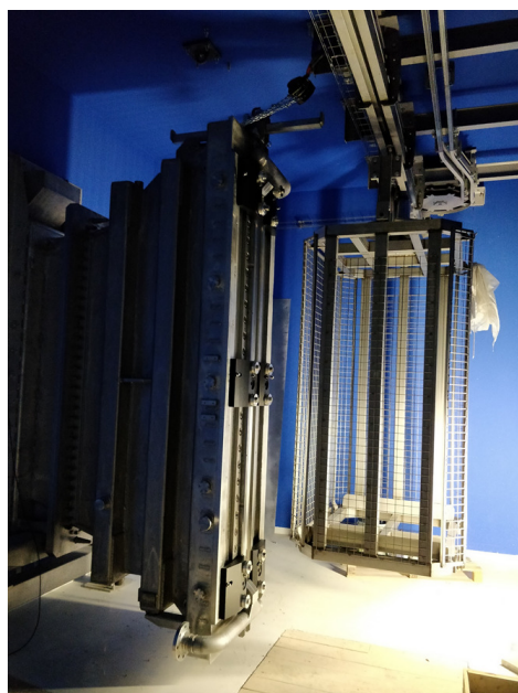
FIGURE 2.7: 5 or 7 MV X-ray scan horn and a pallet conveying system at the feerix ® facility at Aerial. X-ray conversion target measures 2.2 m long and is made of tantalum.
