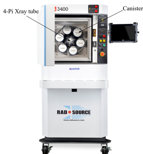
FIGURE 2.10: RS3400 4pi X-ray irradiator[132].
