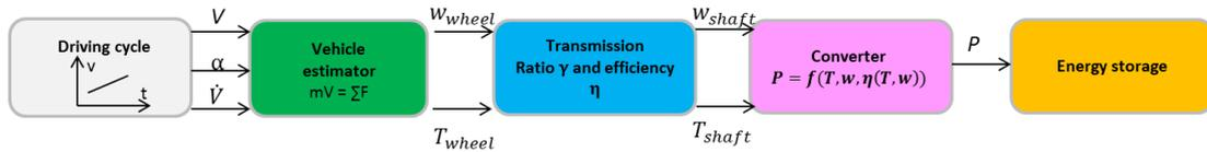
Figure\_B-1: Generic backwards simulation model
