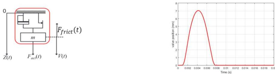
Figure\_ B-11: Mechanical part of the actuator and lift profile Zref to be ensured for a mechanical valve train and an engine speed of 6000 rpm
