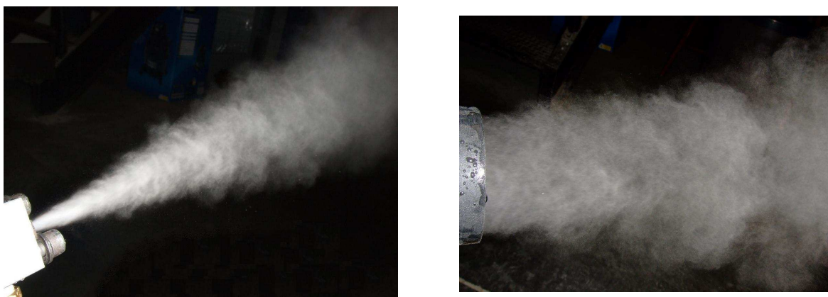
Figure 46. Spray quality of the injector (left) and the air/spray mixer (right)
