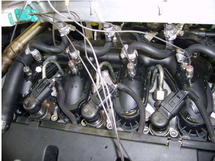
a) Instrumented intake manifold
