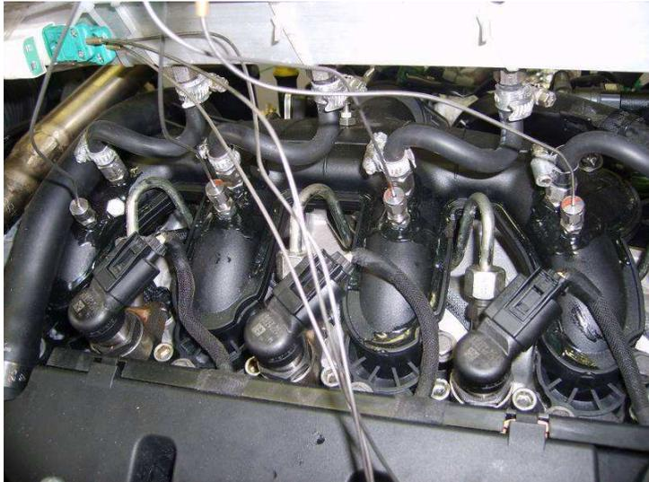
a) Instrumented intake manifold
