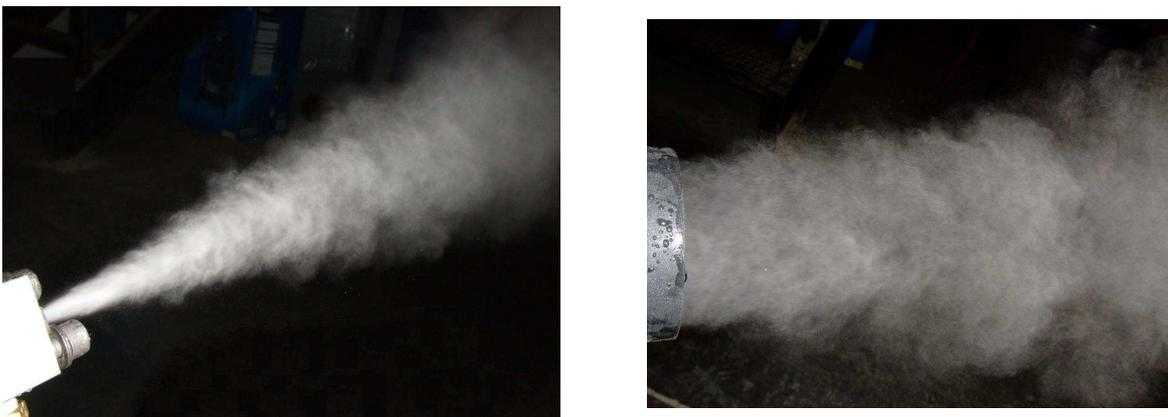
**Figure 46.** Spray quality of the injector (left) and the air/spray mixer (right)
