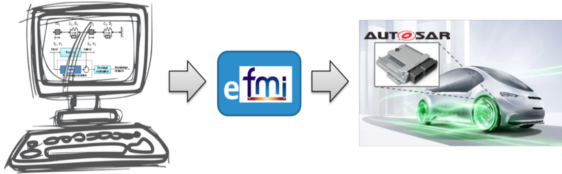
Figure 1.8: Simplified schematic of eFMI workflow [EMPHYSIS 2017]
