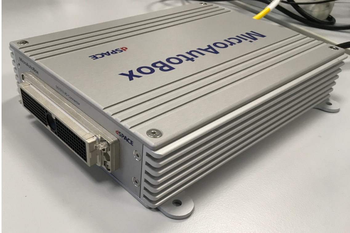
Figure 3.9: dSPACE MicroAutoBox II - 1401/1511
