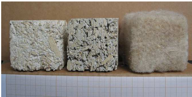
Fig. 6. Samples of lime–hemp render, hemp mortar and hemp wool.
