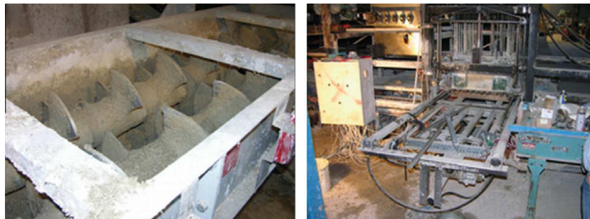
Fig. 2. Precasting method (left: mixer, right: block press).
