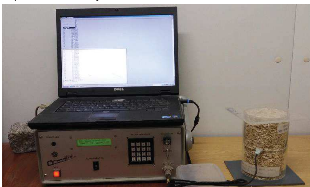
Fig. 5: Experimental device for the measurement of thermal conductivity
