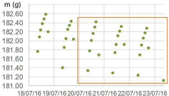
Fig. 14: Moisture uptake and release for sample n°1-A
