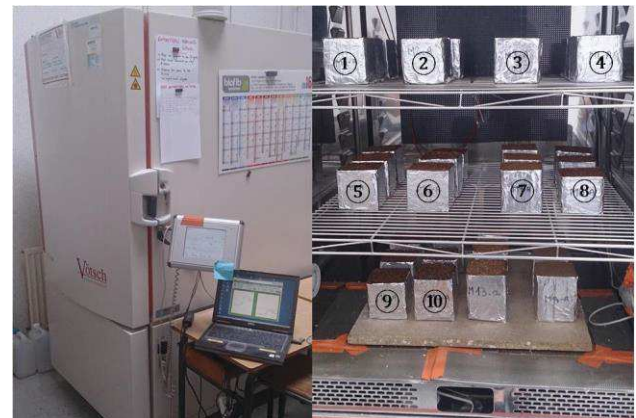
Fig. 8: Experimental device for the measurement of Moisture Buffer Value
