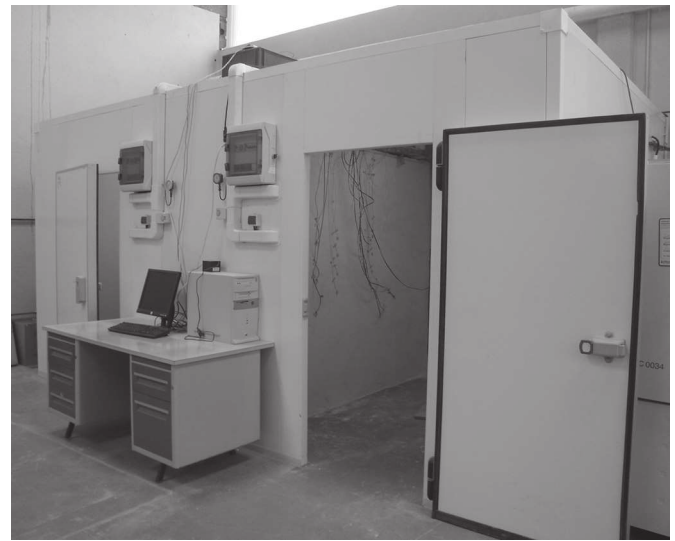
Fig. 1. Experimental device: bi-climatic rooms.
