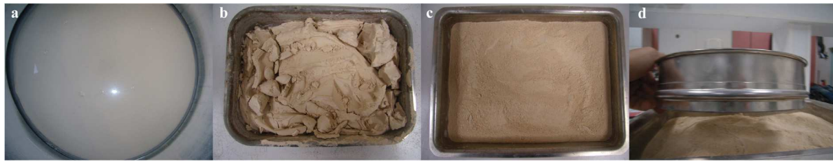
Fig. 1. Preparation of clay binder: a) decanting; b) Drying; c) Milling; d) Sieving with a square mesh of 2 mm.
