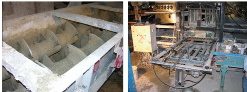
Fig. 2. Precasting method (left: mixer, right: block press).
