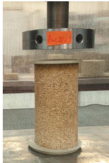
Fig. 11. Compressive test device.
