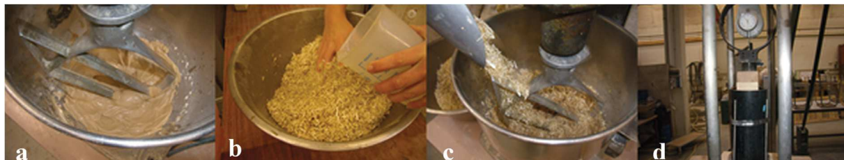
Fig. 8. Production process: a) Binder mixing; b) Hemp mixing by hand; c) Addition of the moist hemp and mixing; d) Compaction.
