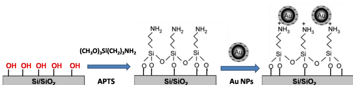
Figure 3.2 Schematic representation of the procedures developed for fabricating gold nanoparticles on the substrate in combination with APTS monolayer.
