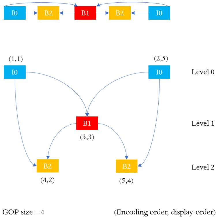
Figure 4.1 Hierarchical B pattern for GOP size = 4
