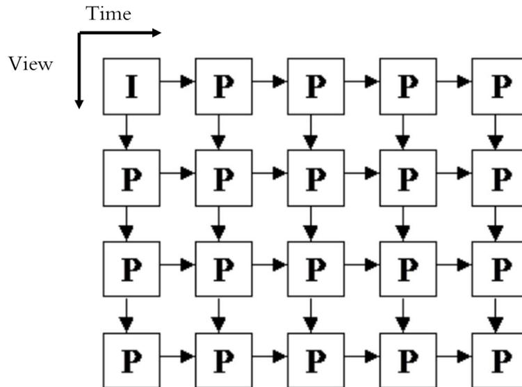
Figure 3.3 Sequential prediction structure [70]
