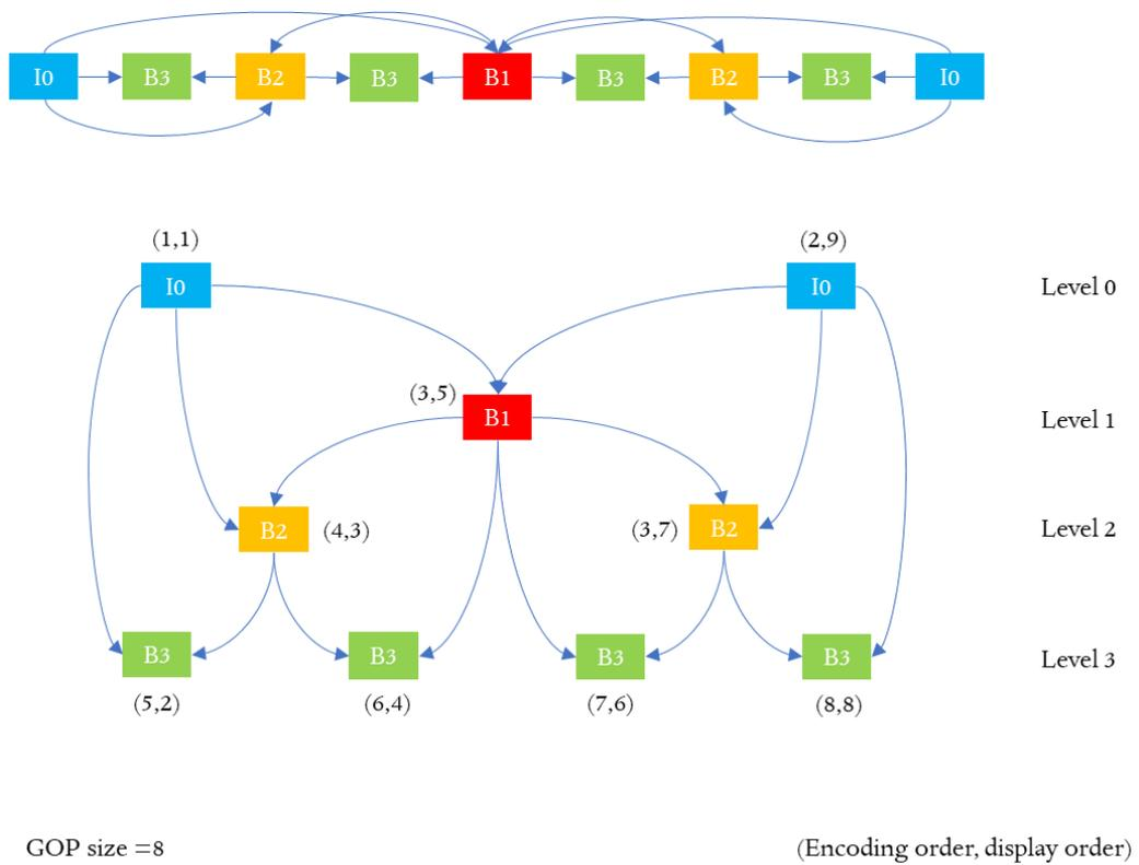
Figure 4.2 Hierarchical B scheme for GOP size = 8
