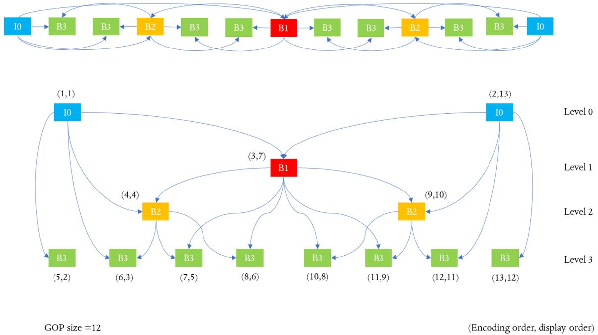
Figure 4.3 Hierarchical B scheme for GOP size = 12
