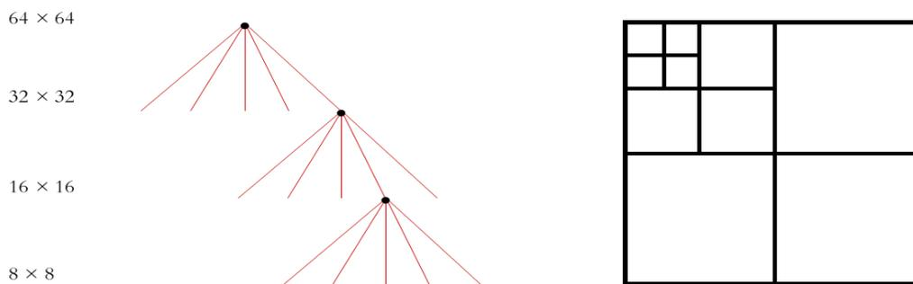
Figure 5.1 CTU partitioning and processing order in HEVC
