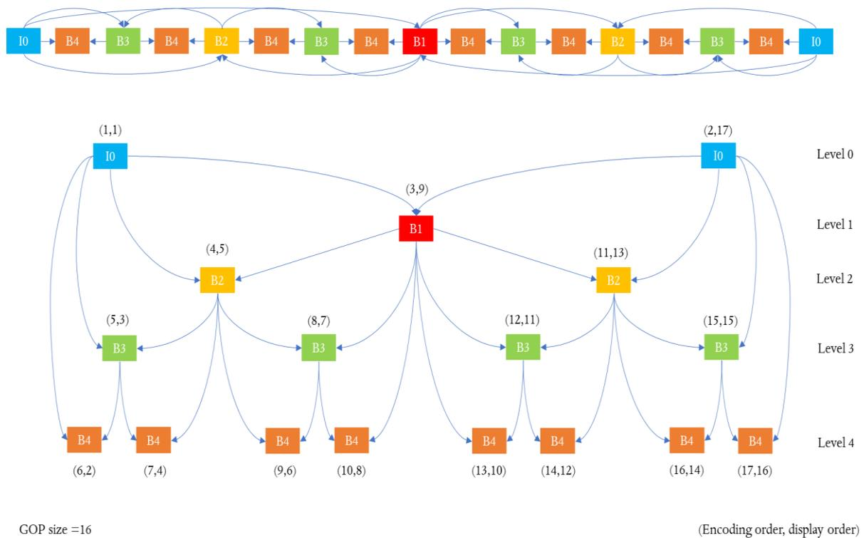
Figure 4.4 Hierarchical B scheme for GOP size = 16
