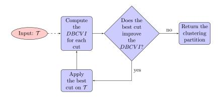
Figure B.3: Diagram summarizing DBMSTCLU algorithm. Figure from [117].
