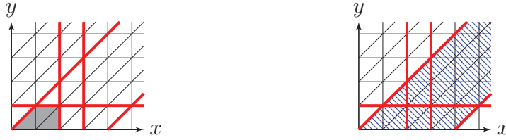
Figure 3.2 – Time successors: the successors of the gray zone on the left are the union of all blue dashed zones on the right.
