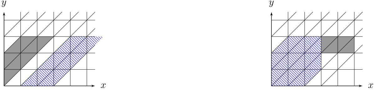
Figure 1.7 – For e = (\ell, g, a, R, \ell') with \text{Inv}(\ell) = \text{Inv}(\ell') = x \leq 6 \wedge y \leq 3 , g = x \geq 1 \wedge y \geq 1 and R = \{y\} , left figure represents in blue the successor of the gray zone by \text{Post}_e . On the right, the blue zone is the predecessor of the gray zone by \text{Pre}_e .
