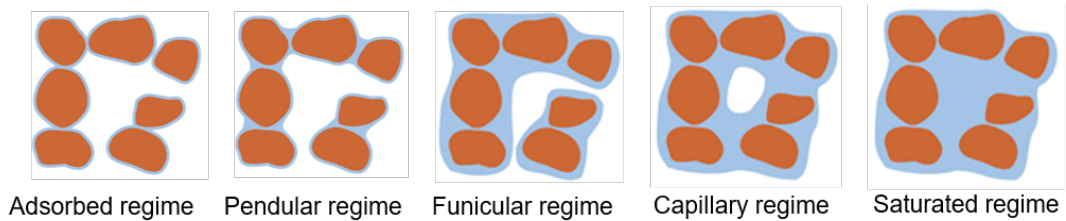
Figure I.7 – Saturation regimes in porous medium showing spatial configurations of air and water. Adapted from Szymkiewicz [22].
