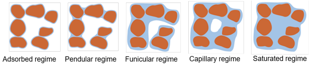
Figure I.7 – Saturation regimes in porous medium showing spatial configurations of air and water. Adapted from Szymkiewicz [22].
