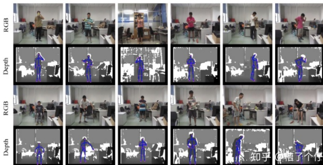
Figure 2.25: Snapshots of activities in SYSU 3D HOI set, one sample per class. The rows headed with RGB show the samples in RGB channel and the rows underneath headed with Depth show the corresponding depth channel superimposed with skeleton data. Best viewed in color.
