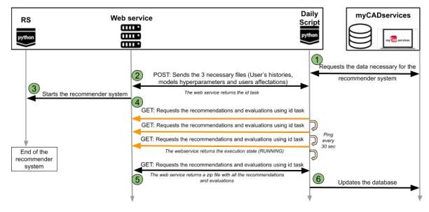
Figure 5.2: Overview of the exchanges between the different components during the daily task.
