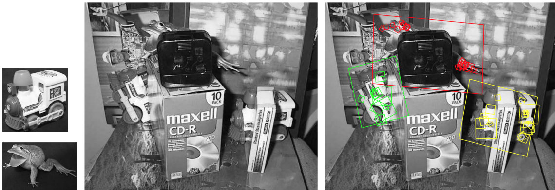
Figure 2.12 – Application of SIFT. (Left) The training images for two objects. – (Middle) These can be recognized in a cluttered image with extensive occlusion. – (Right) The results of recognition. A parallelogram is drawn around each recognized object, showing the boundaries of the original training image under the affine transformation solved for during recognition. Figure reproduced and caption from (Lowe 2004).
