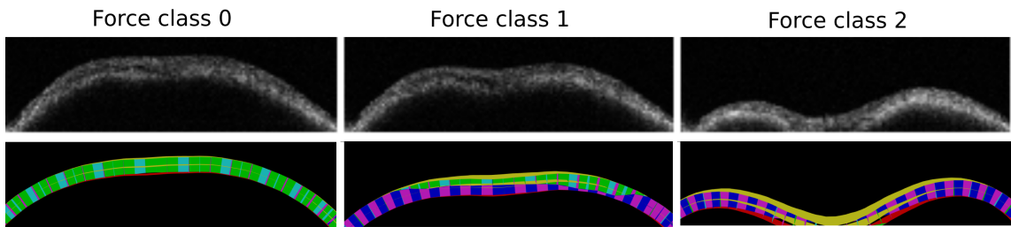
Figure 6.6: Real OCT images of the eye used for the data assimilation and matching simulated images with E = 0.25 \text{ MPa} for the three force ranges.
