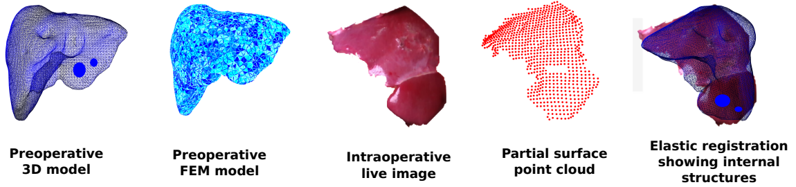
Figure 7.1: Augmented reality pipeline: preoperative internal structures are mapped in real-time onto the live image of the organ using a FEM model.
