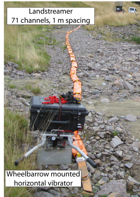
Fig. 3. Pictures depicting S-wave seismic reflection acquisition using wheelbarrow mounted horizontal seismic vibrator with landstreamer along the gravel path for profile 4.
