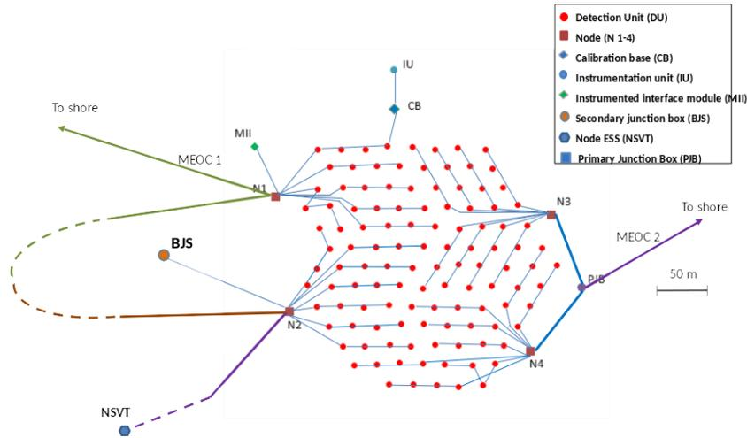
Figure 2.3: Seafloor layout of the KM3NeT ORCA detector.
