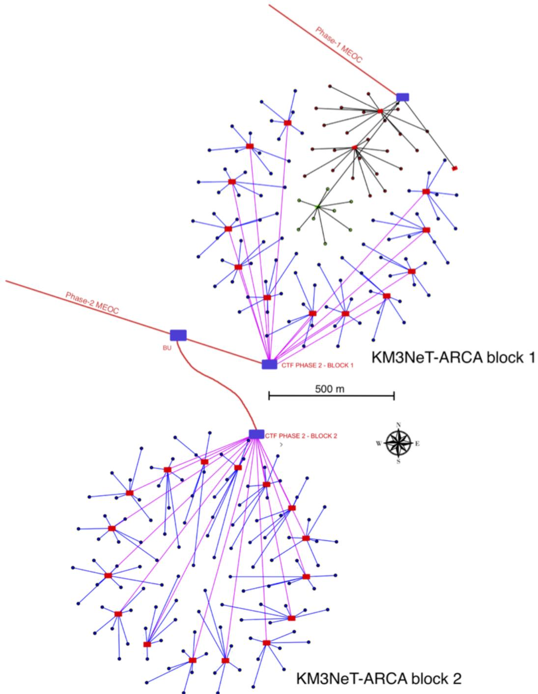
Figure 2.2: Seafloor layout of the KM3NeT ARCA detector. The *Phase-1* represents the first construction milestone. Source: [126].
