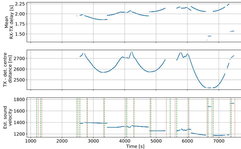
Figure 5.10: Mean delay between reception times and emission time (top), distance between the transmitter and the center of the detector (middle) and corresponding estimated sound velocity (bottom) as a function of the emission time of the chirp. On the bottom panel, the vertical green and red lines indicate the start and end time of each segment (cf. Figure 5.5).
