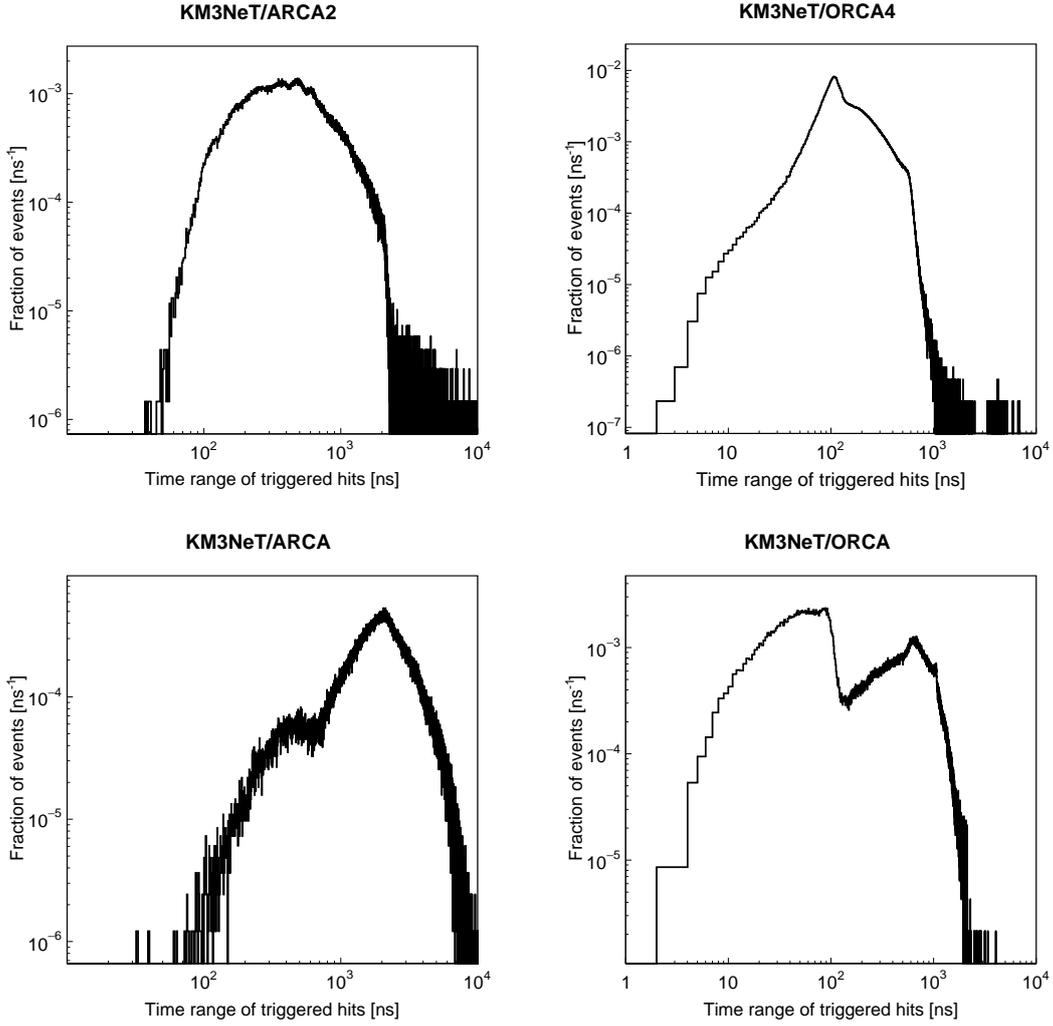
Figure 4.13: Time range of triggered hits for sea data of ARCA2 and ORCA4 (top) and simulated data of ARCA and ORCA (one building block). The two populations visible for the 115-lines detectors come from the shower and track triggers, respectively.
