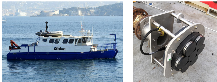
Figure 5.4 – The GG9 vessel (left) and the ECHOES 10000 hydroacoustic transducer (right).
