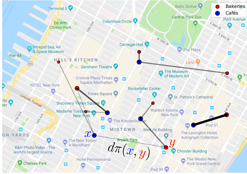
Figure 2.2: The bakery/cafés problem in Manhattan based on example 2.1.2. The bakeries ( resp cafés) are in blue ( resp red) and the dots' size denote the amount of bread disposable ( resp needed). Lines represent the amount of bread transferred d\pi(x, y) : the wider the larger. The optimal transport plan is depicted in the Figure and represents the cheapest transport plan so that all breads are transferred from bakeries to cafés.
