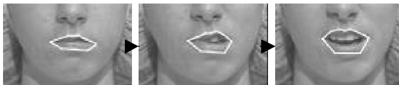
Figure 3.3 – Mouth segmentation from a sample of AU-Coded Facial Expression Image Database (Kanade et al., 2000).
