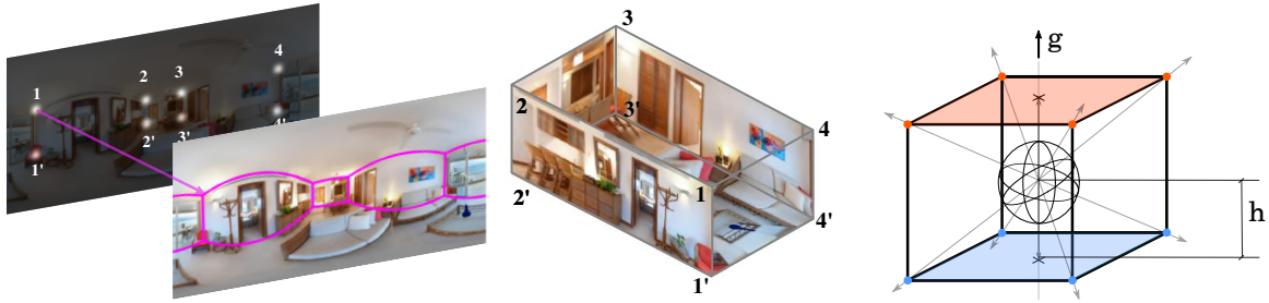
(a) The 2D corners coordinates are the maximum activations in the probability map. From the 2D corners, we can directly recover the 3D layout by doing a couple of assumptions.
