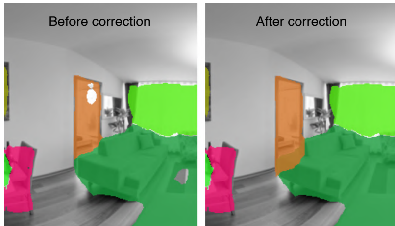
Fig. 3.5 After combining the room layout with our segmentation masks, the model experiences a clear improvement as a whole. However, here we want to show a failure case where, when assuming that doors must reach the floor, we may have overlapping with other occluding objects in the image, damaging segmentation results but improving the door 3D localization.
