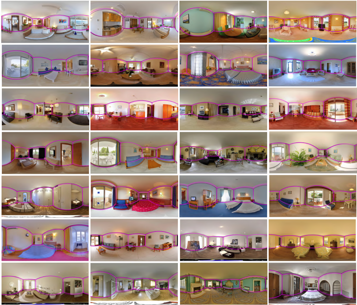
Fig. 2.25 Layout predictions (light magenta) and ground truth (dark magenta) on the SUN360 annotation dataset [157]. Best viewed in color.
