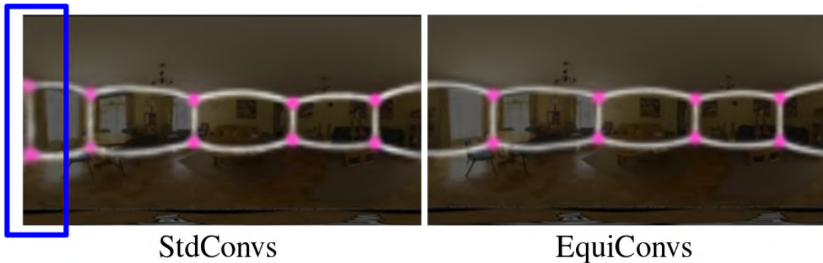
Fig. 2.19 EquiConvs show more consistent qualitative results whereas StdConvs simply do not understand that the image wraps around the sphere, losing the continuous context that these images provide.
