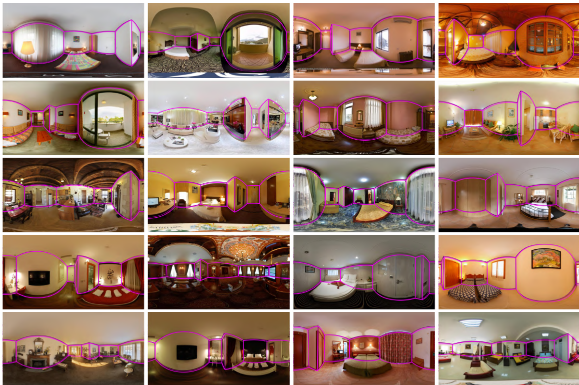
Fig. 2.26 Layout predictions (light magenta) and ground truth (dark magenta) for complex room geometries on the SUN360 annotation dataset [157]. Best viewed in color.
