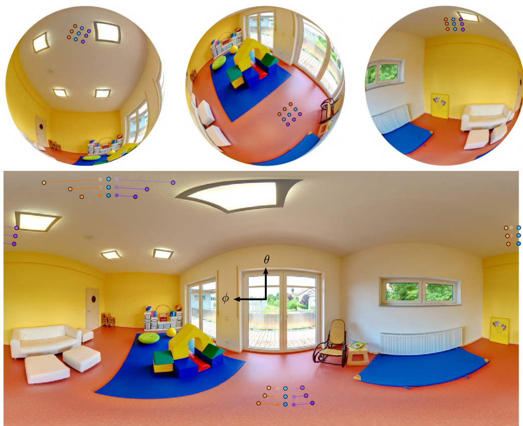
Fig. 2.16 EquiConvs on spherical images. We show three kernel positions to highlight the differences between the offsets. As we approach to the poles (larger \theta angles) the deformation of the kernel on the equirectangular image is bigger, in order to reproduce a regular kernel on the sphere surface. Additionally, with EquiConvs, we do not use padding when the kernel is on the border of the image since offsets take the points to their correct position on the other side of the 360^\circ image.
