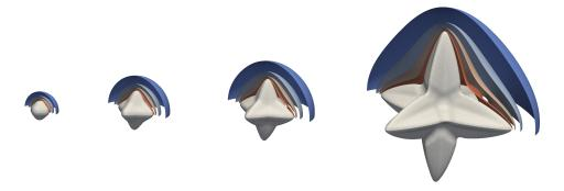
Figure 4.1: Evolution of the shape of an equiaxed grain envelope and of the concentration field around the envelope. Iso-surfaces of concentration are shown.
